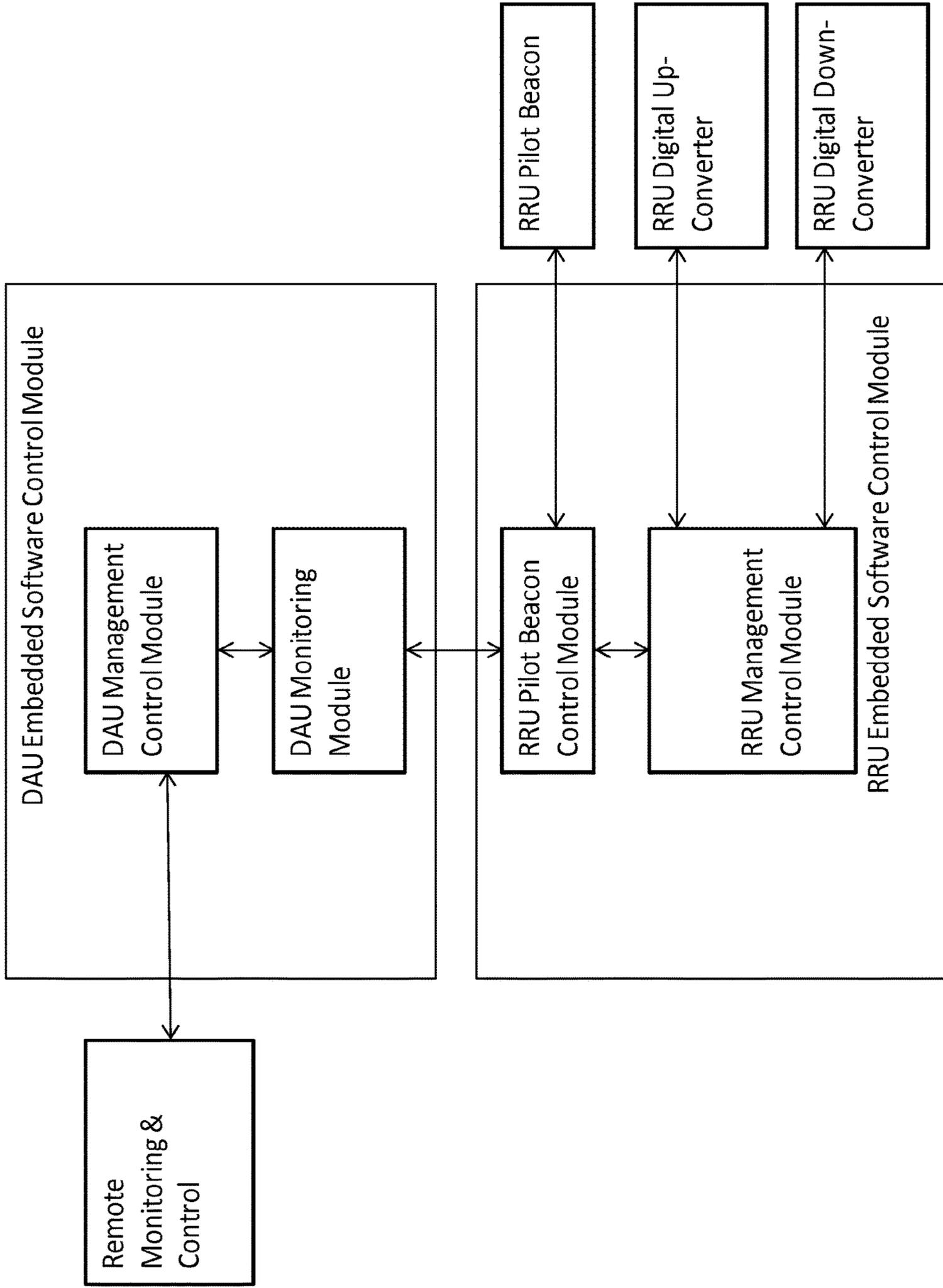
Figure 7: Embedded Software Control Modules
