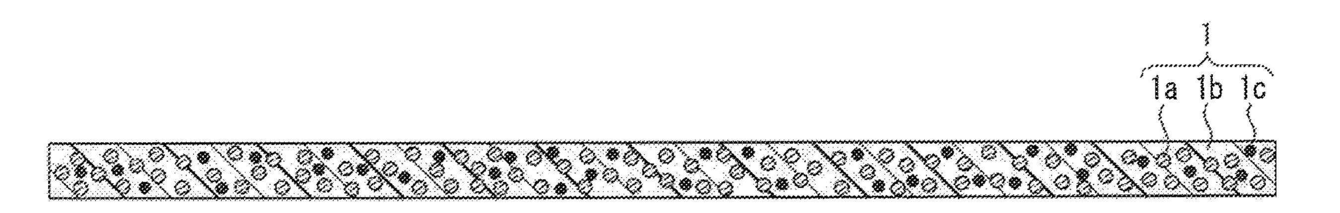
nates in a frequency band in or above a millimeter-wave band as an electromagnetic-wave absorbing material 1a, and is a nonresonant-type electromagnetic-wave absorber that is not provided with a reflective layer for reflecting incident electromagnetic waves.
