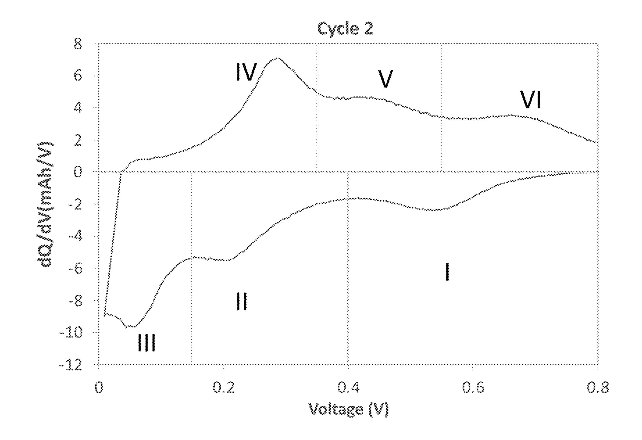
**Figure 3.** Differential capacity vs voltage plot for Silicon-Carbon Composite 3 from 2<sup>nd</sup> cycle to 5<sup>th</sup> cycle using a half-cell.
