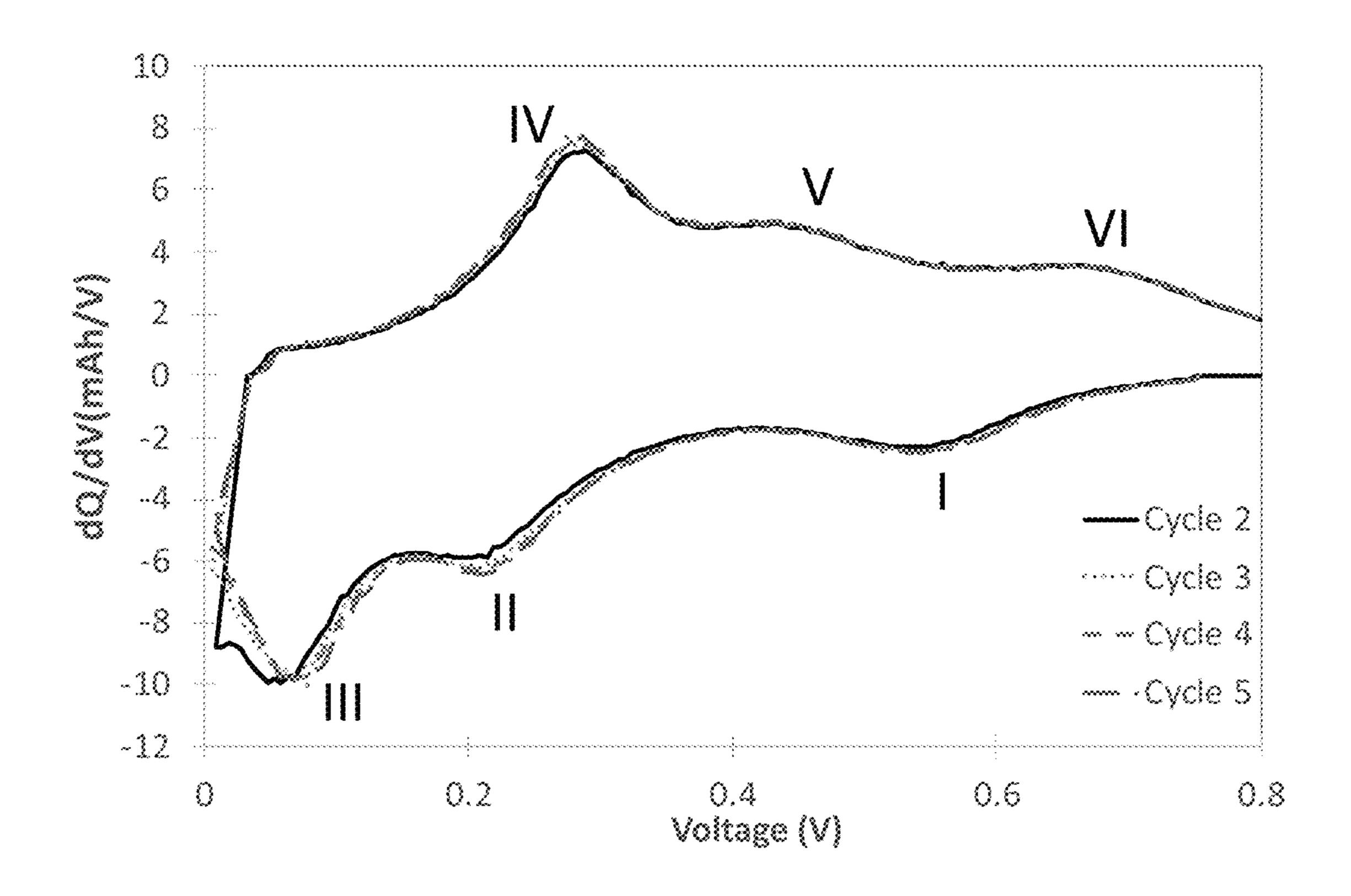
Figure 4. dQ/dV vs V plot for various silicon-carbon composite materials.
