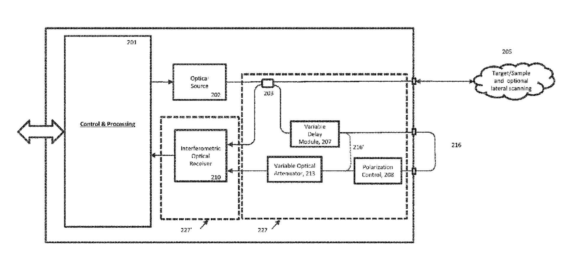
is configured to generate an interferometric measurement signal based on the receive signal.
