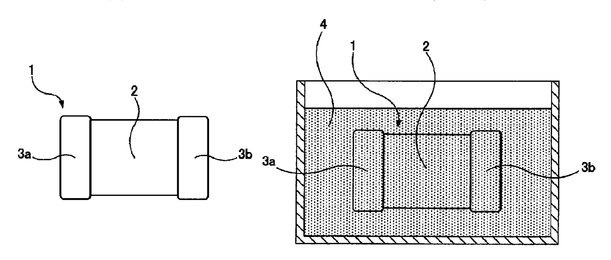
be coated with the coating material. The selected surface material has different material properties than the non-selected surface material. The element body is coated with the coating material by applying a surface modifier only on the surface of the selected surface material and thereafter coating the surface of the selected surface material to which the surface modifier has been applied with the coating material.
