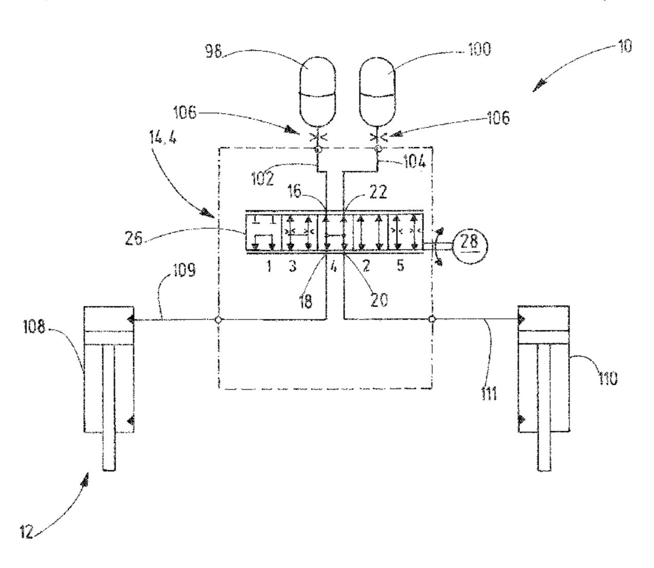
valve piston (26), the axle oscillation is provided while the suspension is blocked and, in at least one further second functional position of the valve piston (26), the suspension is provided while the axle oscillation is blocked.
