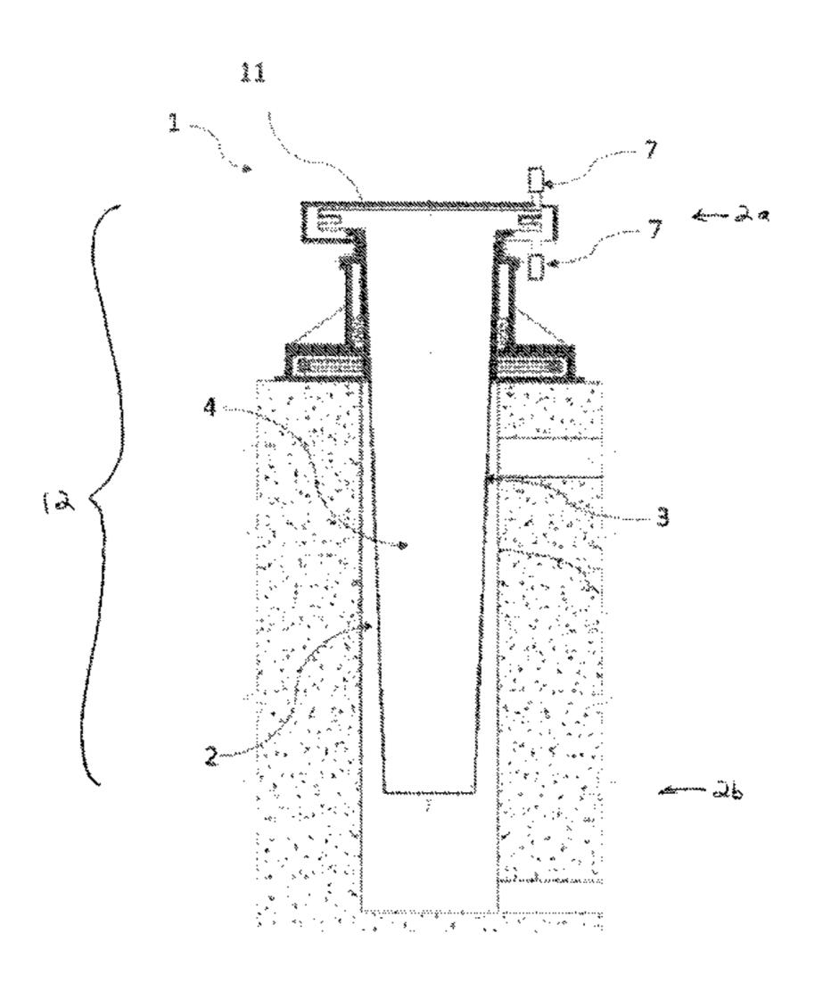
reaction; movement means configured to rotate the casing about the central axis and to force the first coolant fluid to contact the wall at the active layer for cooling the casing; and external cooling including a second coolant fluid contacting at least an external portion of the wall.
