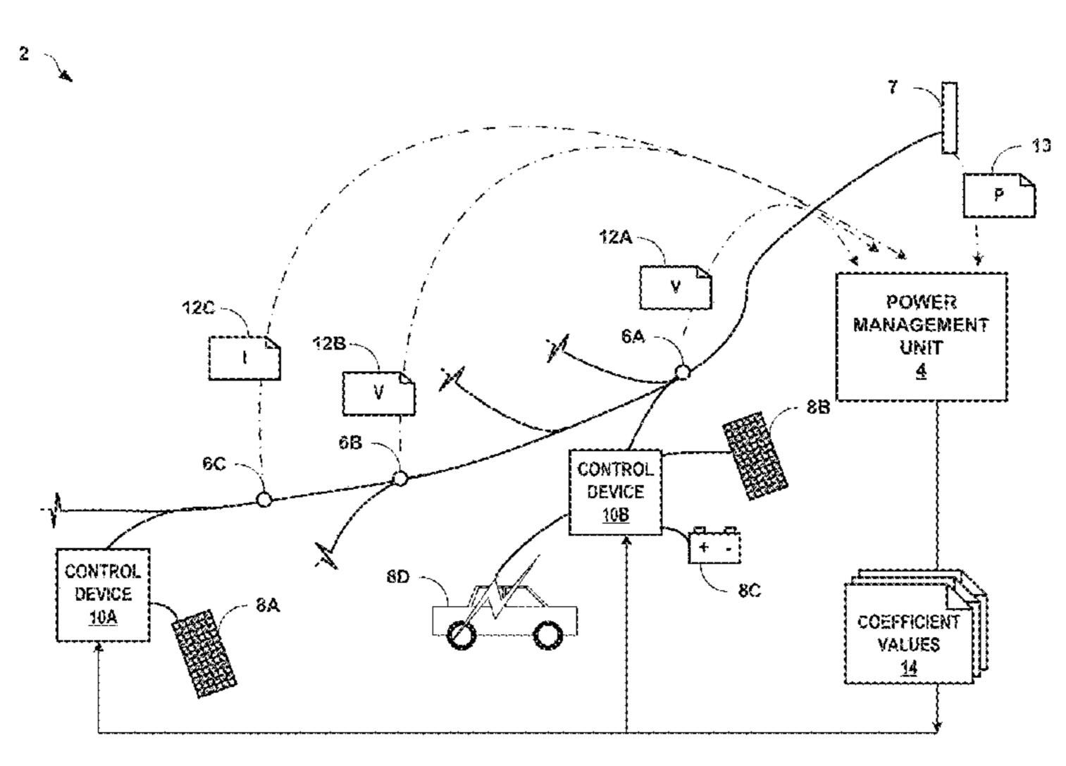
system and determine for the connection point, a respective value of first and second power-constraint coefficients. The processor is also configured to cause at least one energy resource connected to the first portion of the power system to modify an output power of the at least one energy resource based on the value of the first and second voltage-constraint coefficients for each voltage node and the value of the first and second power-constraint coefficients.
