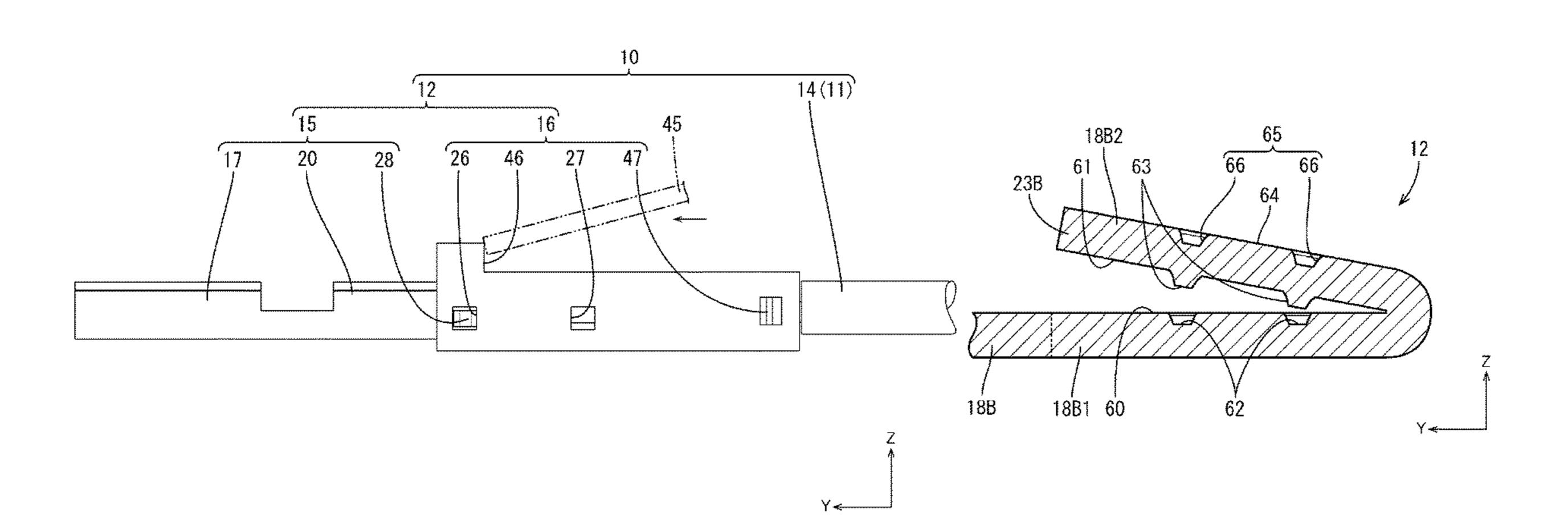
the overlapping portion and a second facing surface of the tip portion are facing each other and overlapped.
