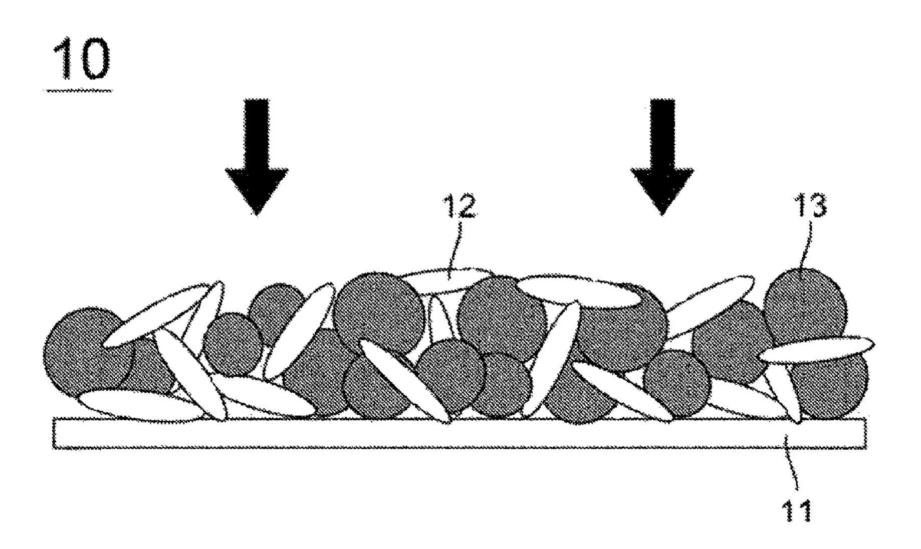
diameter ( $D_{50}$ ) of the scaly natural graphite is 10  $\mu m$  to 15  $\mu m$  and an average particle diameter ( $D_{50}$ ) of the spherical natural graphite is 14  $\mu m$  or less.
