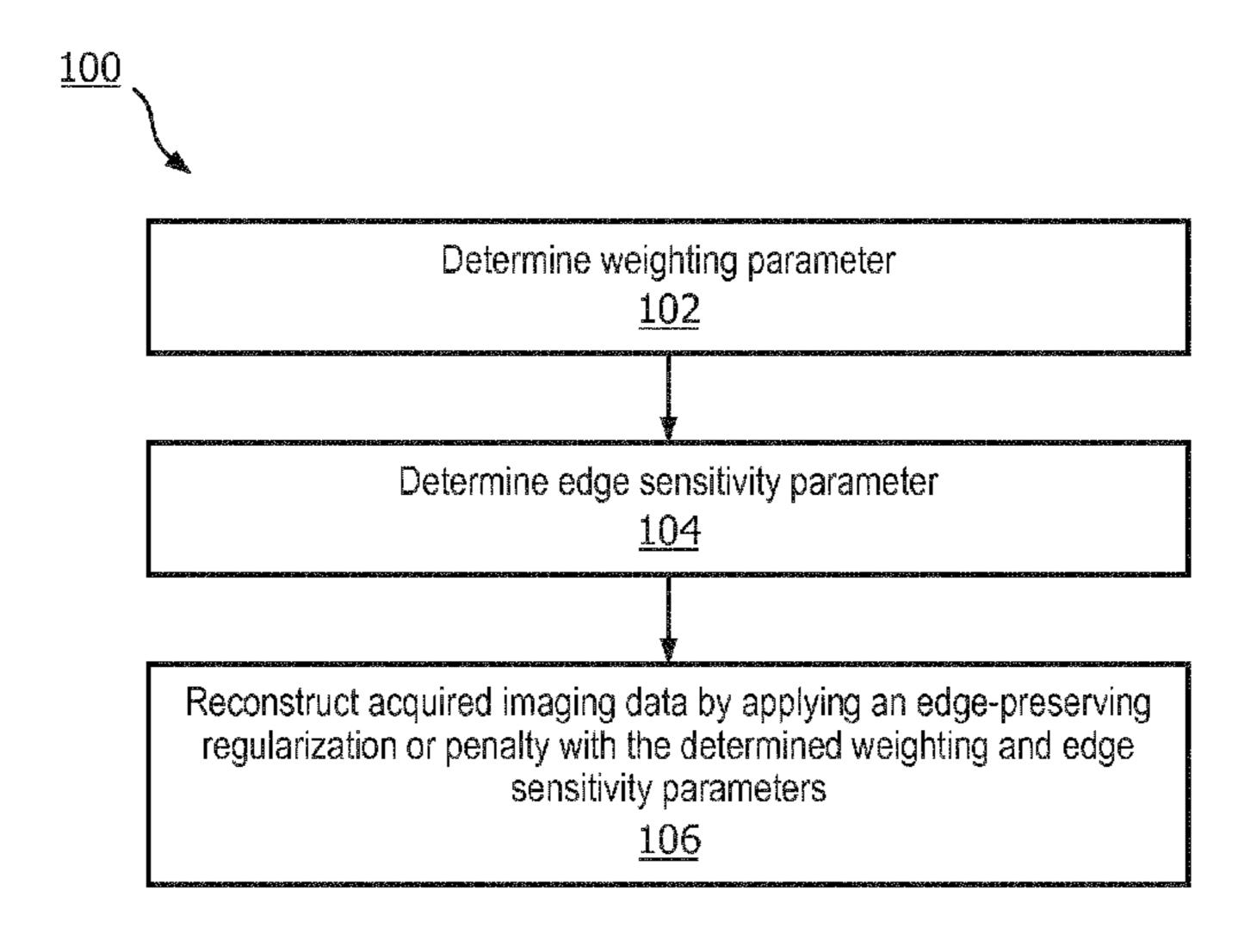
acquisition device; and reconstructing the imaging data set obtained by the image acquisition device to generate a reconstructed image by applying the regularized image reconstruction including the edge-preserving regularization or penalty with the determined weighting and edge sensitivity parameters to the imaging data set obtained by the image acquisition device.
