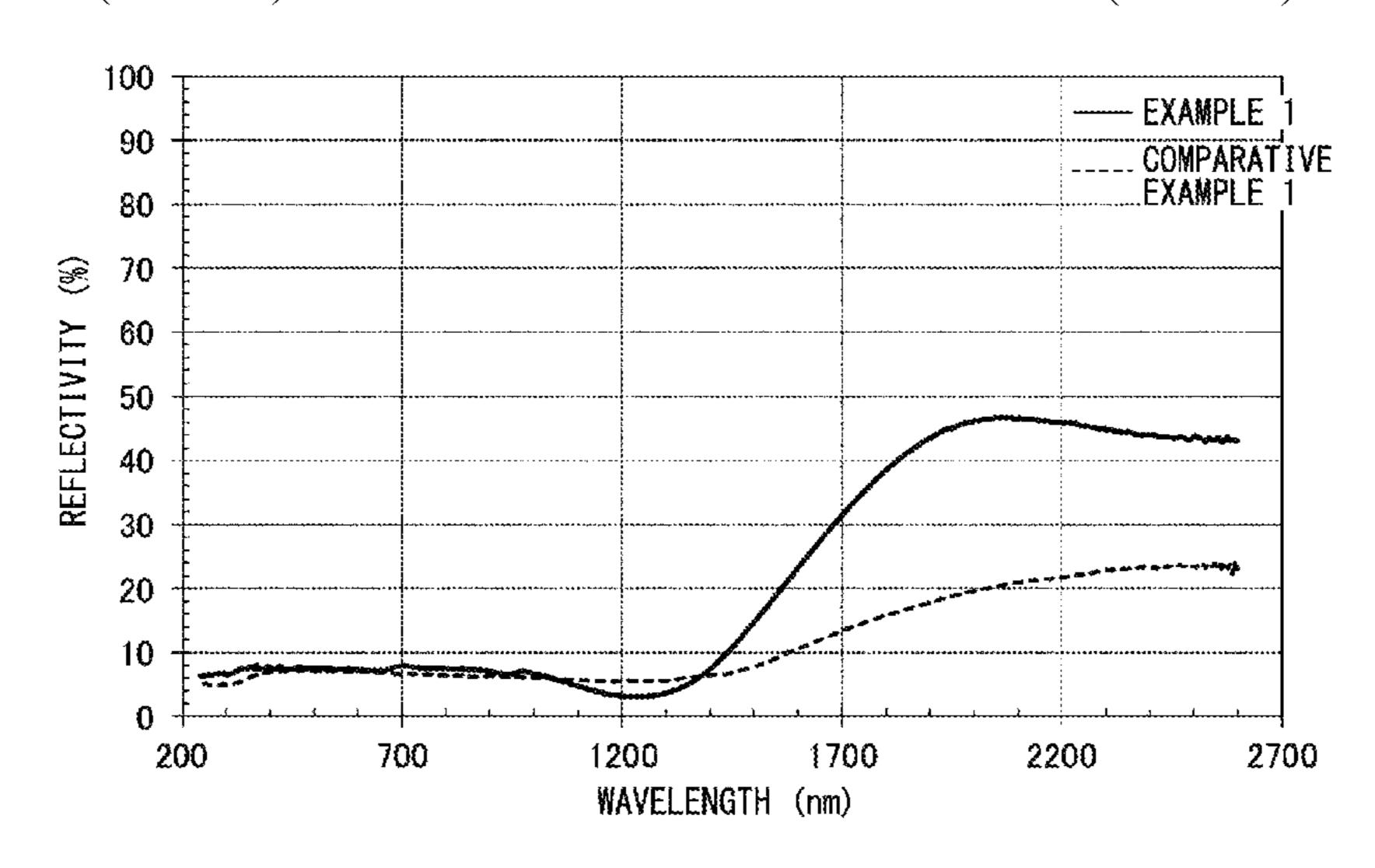
infrared-shielding film, the metal oxide microparticles are dispersed in a hydrophobic solvent, and a light transmittance in a wavelength range of 800 nm to 1,100 nm is 20% or more and less than 70%.
