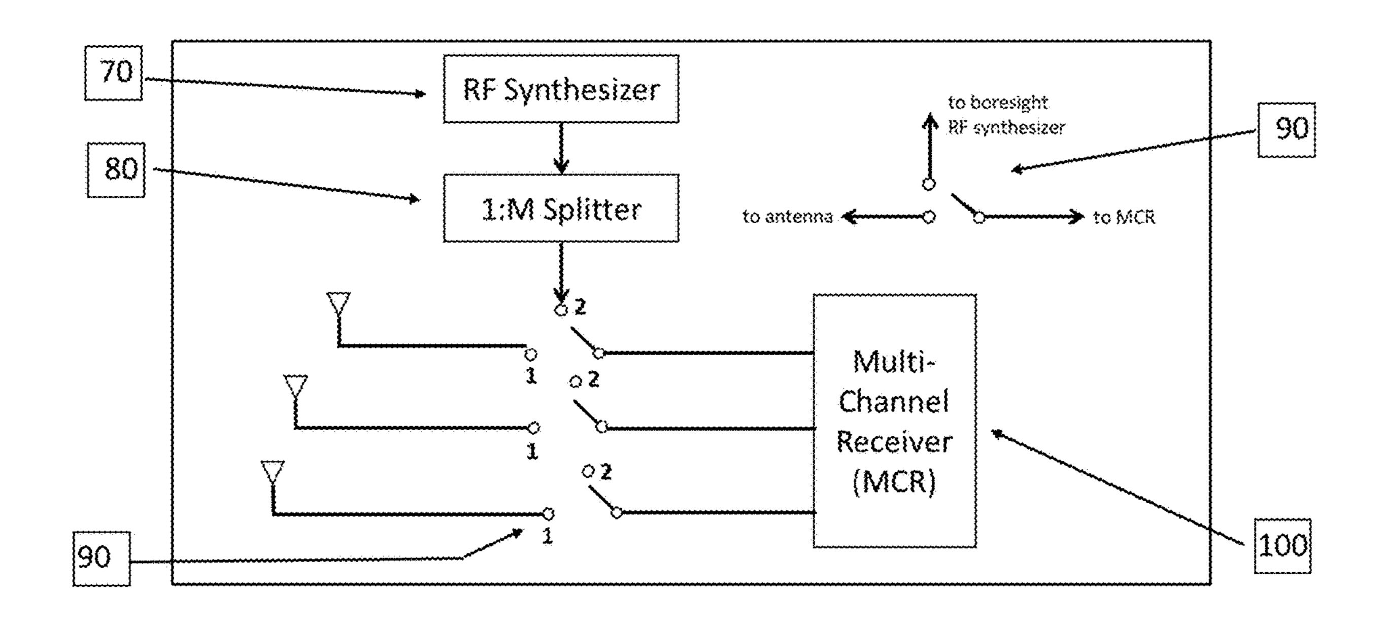
RF Synthesizer path produces the boresighting signal
