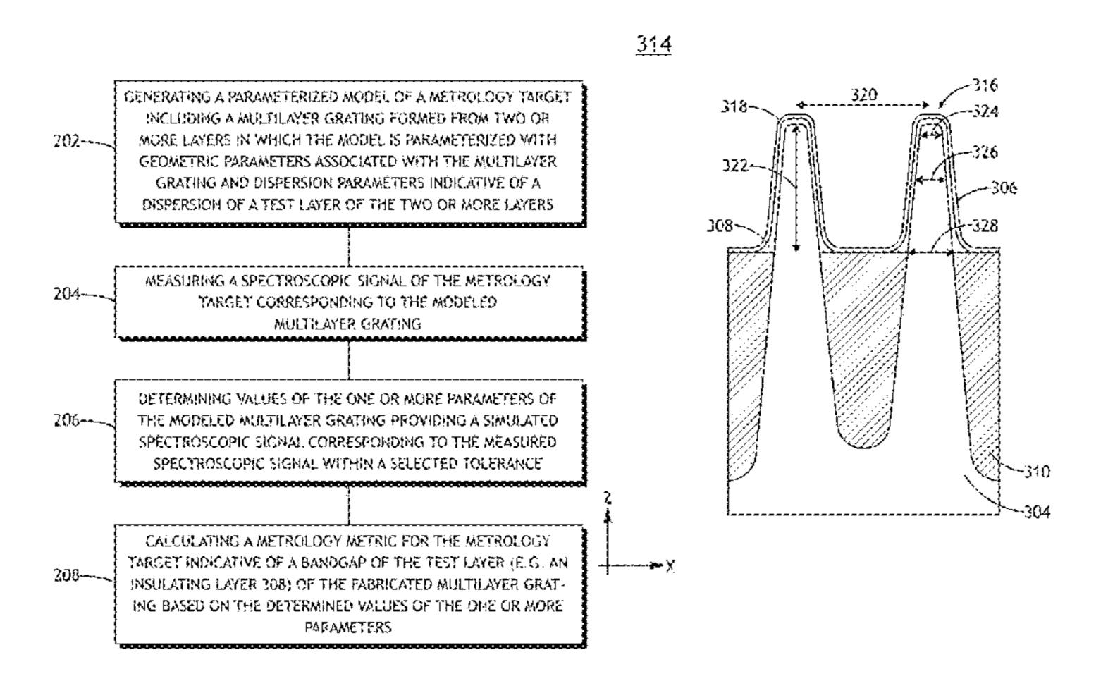
viding a simulated spectroscopic signal corresponding to the measured spectroscopic signal within a selected tolerance. The controller further predicts a bandgap of the test layer of the fabricated multilayer grating based on the determined values of the one or more parameters of the test layer of the fabricated structure.
