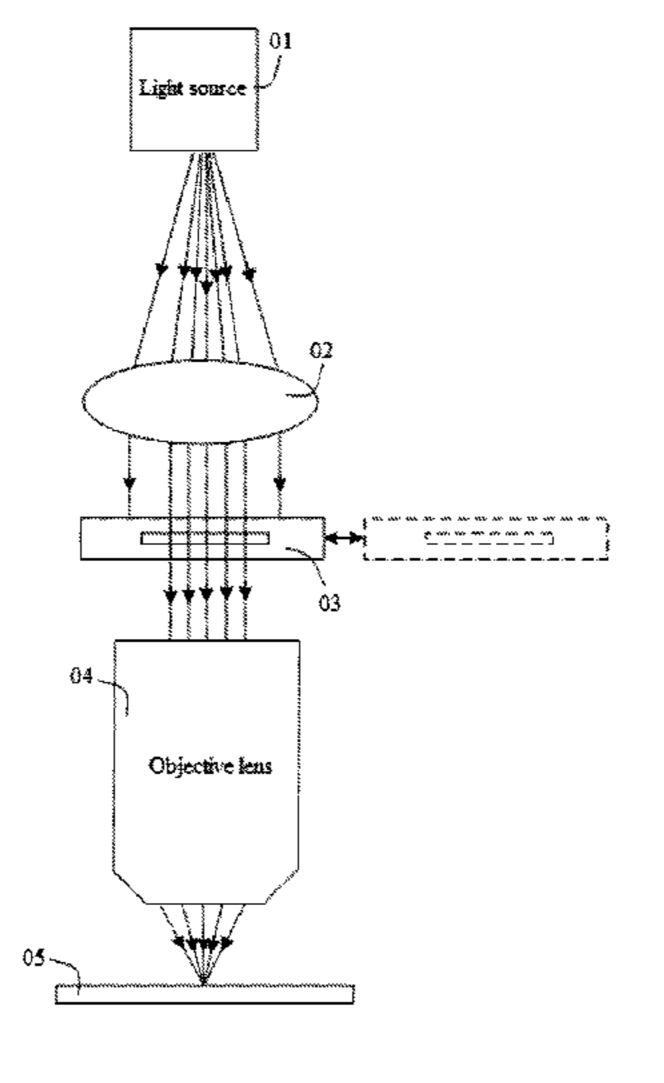
high aspect ratio structure so as to block a portion of light having a large included angle with the normal direction of the object to be tested (05).
