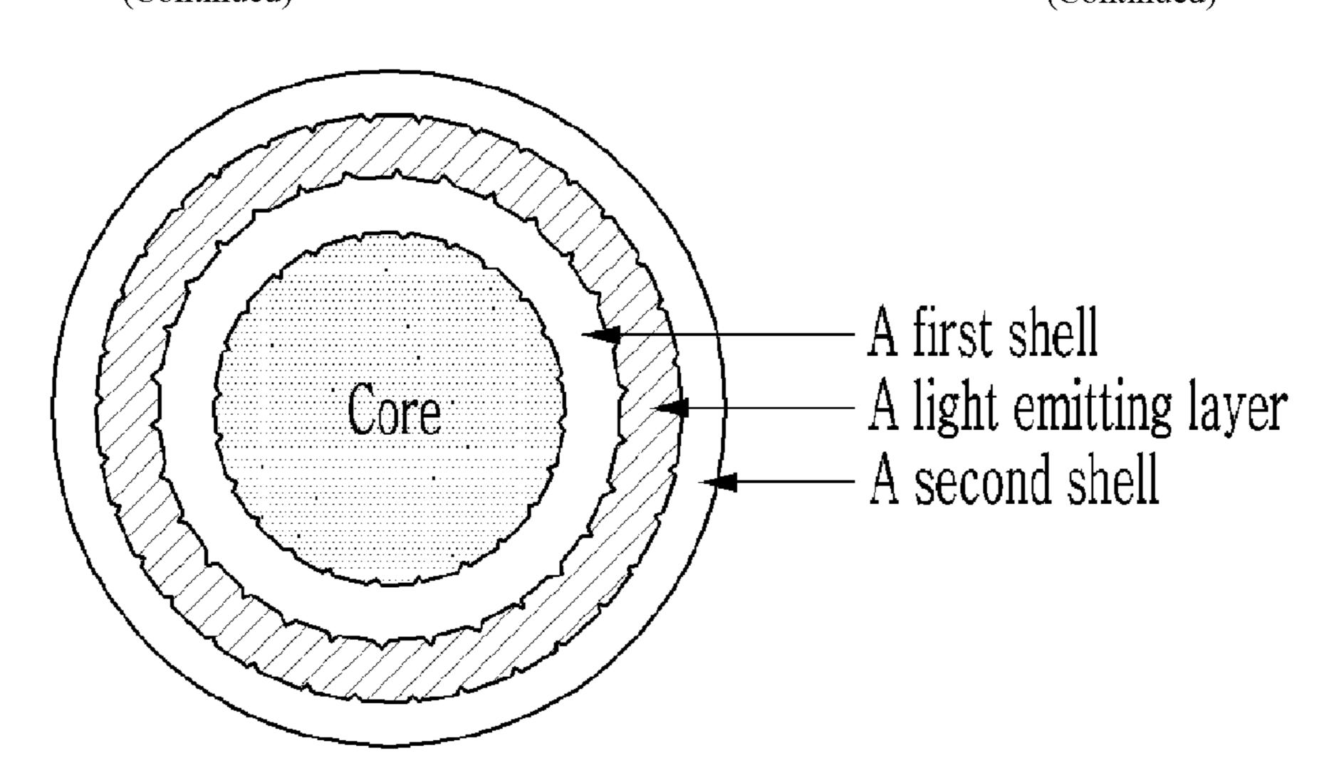
thereof; and a second shell disposed on the light emitting layer and including a semiconductor nanocrystal including zinc, and selenium, sulfur, or a combination thereof, and wherein the quantum is a single light emitting quantum dot having an emission peak wavelength in a range of about 500 nanometers (nm) to about 550 nm.
