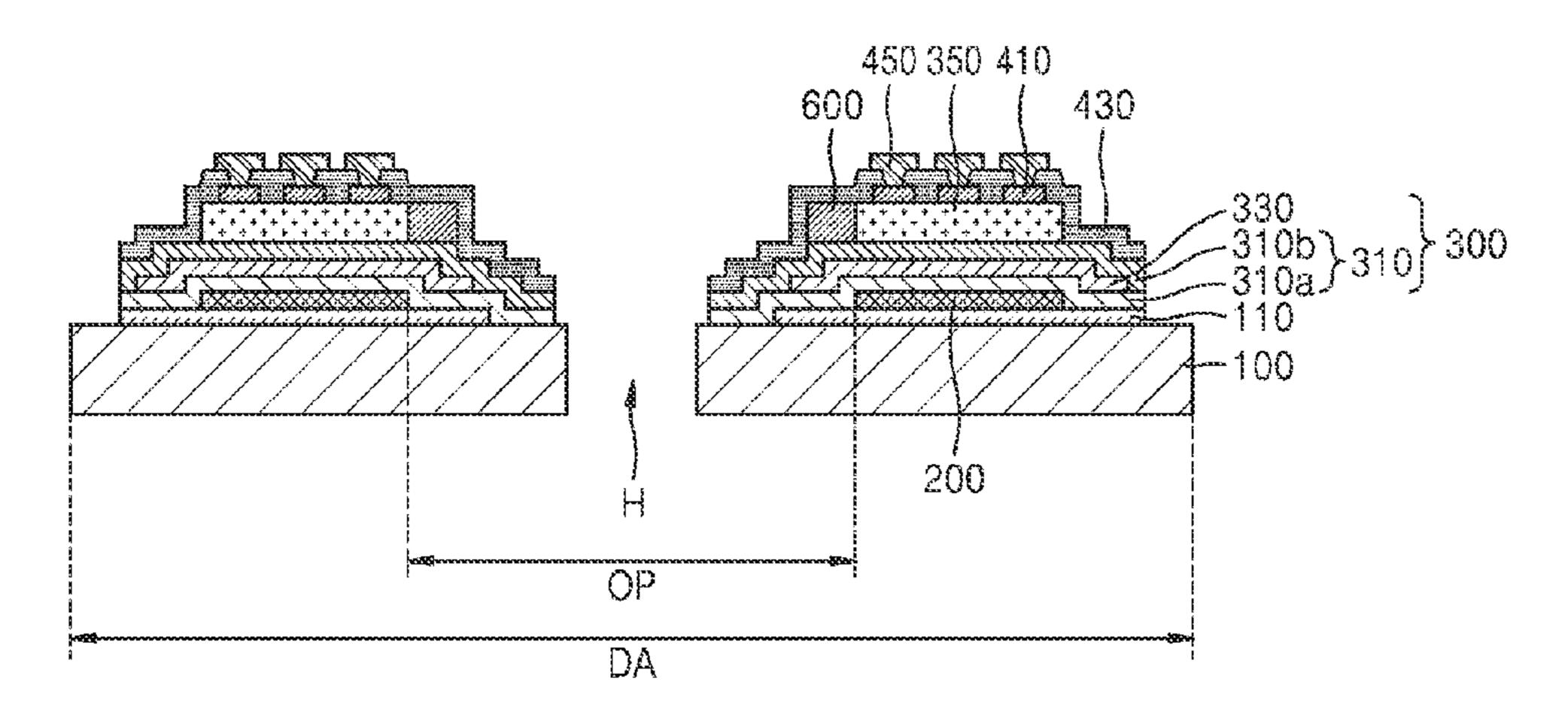
formed over the substrate in the opening portion, forming a touch contact hole by removing a portion of the touch insulating film to expose a portion of the touch electrode, and removing a portion of the touch insulating film and a portion of the thin film encapsulation layer formed in the opening portion to expose a portion of the substrate during the forming of the touch contact hole.
