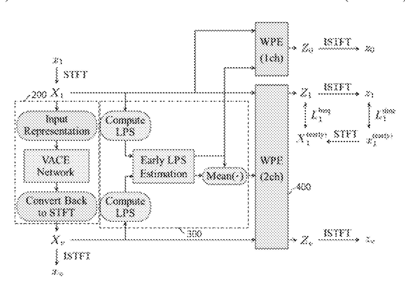
the first speech signal and a dereverberation unit for removing reverberation of the first speech signal and generating a dereverberated signal from which the reverberation has been removed by applying a dual-channel weighted prediction error (WPE) algorithm based on a deep neural network to the first speech signal and the second speech signal.
