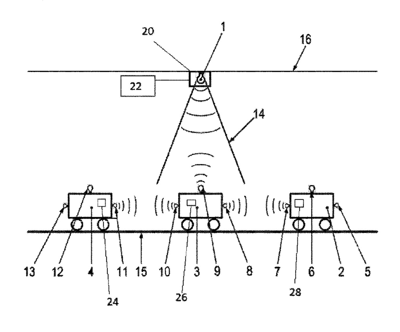
second vehicle transmits data via the first vehicle and the stationary transceiver module to the central control unit.
