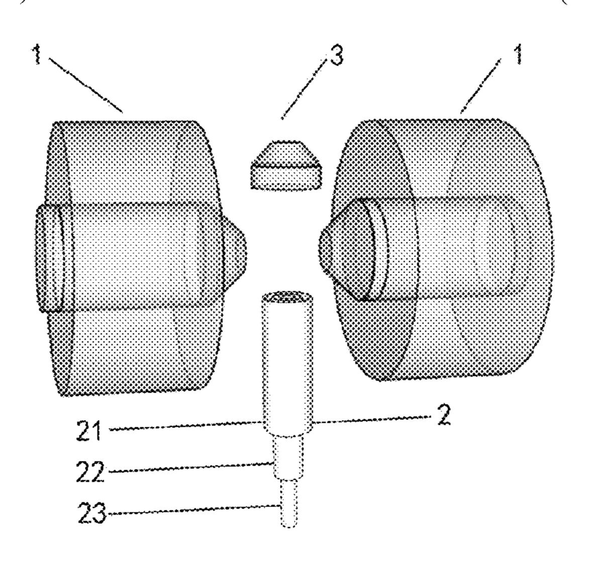
buoyancy lift effect, so that flame synthesis is carried out under a simulated zero/microgravity flame to prepare the nanoparticles. The device is able to use a gradient magnetic field to simulate the zero/microgravity flame on the ground to synthesize the nanoparticles under special flame characteristics, with reduced flame disturbance, improved stability, and no overheated region.
