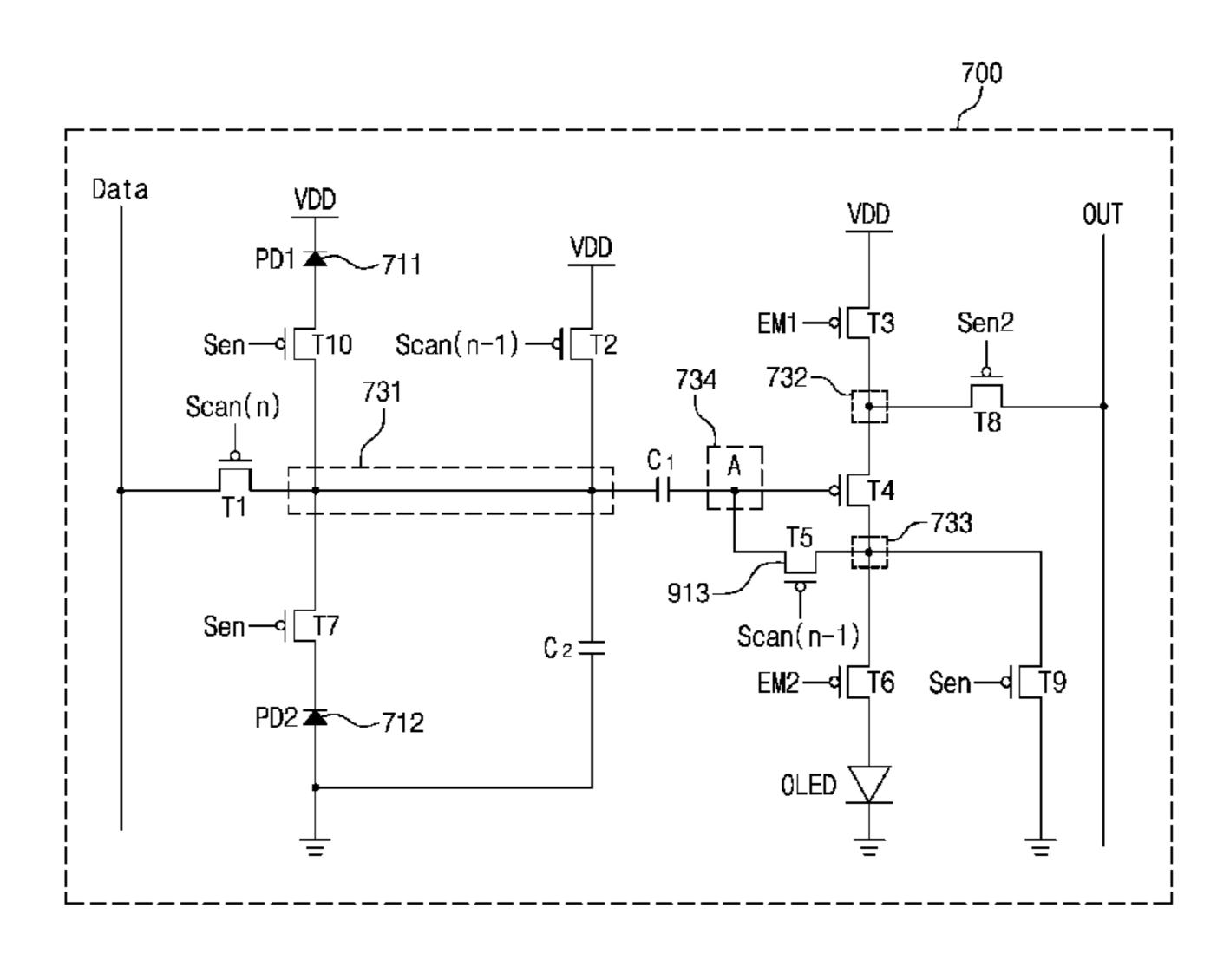
sensing circuit comprises a pixel control circuit, the pixel control circuit comprising: a first photodetector which receives a light and generates a first signal; a second photodetector which receives a light and generates a second signal; and a self-illuminator which receives differential signals of the first signal and second signal and outputs an output signal, includes at least one transistor component and at least one capacitor component, and outputs a light on the basis of a data signal.
