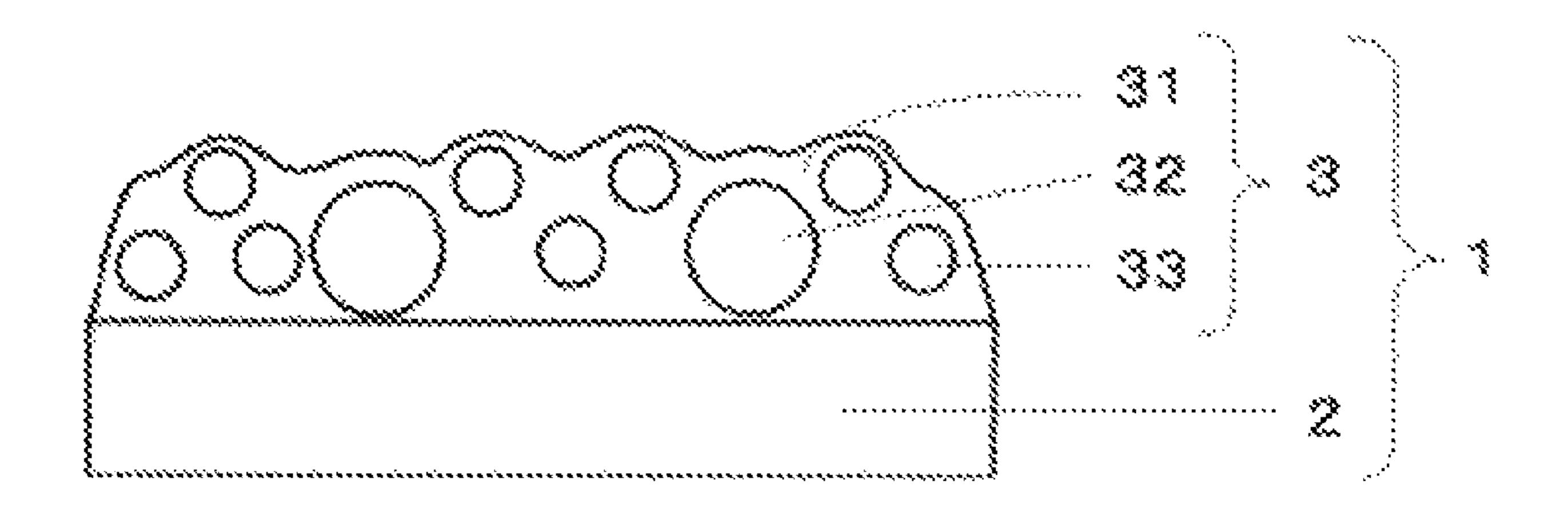
preferably 0.01 to 0.3  $\mu m$ . The optical density of the light-blocking membrane (3) is preferably 0.54 to 2.00  $(\mu m^{-1})$  in terms of thickness.
