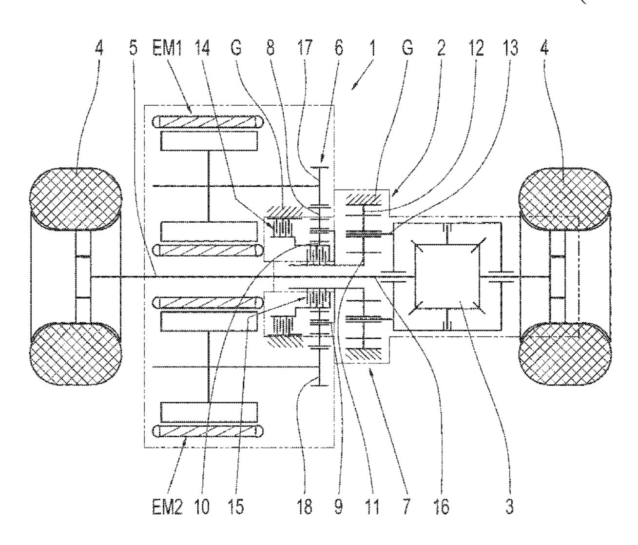
A carrier of the first planetary gear set is rotationally fixed to a sun gear of the second planetary gear set. A sun gear of the first planetary gear set is detachably couplable to a housing. A ring gear of the second planetary gear set is coupled to the housing. A carrier of the second planetary gear set is an output of the transmission. The first planetary gear set is interlockable.
