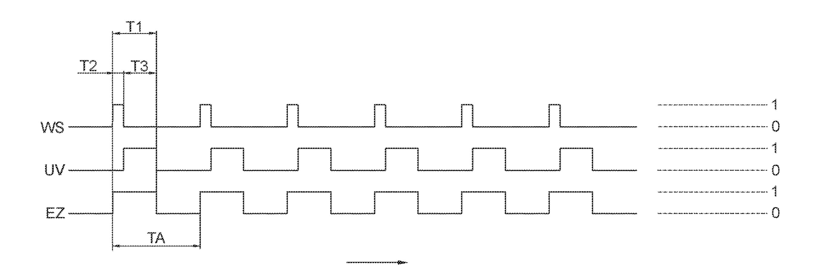
cally mapping the portion, to white light and either to UV light or to IR light during the duration of the on-time of the line camera.
