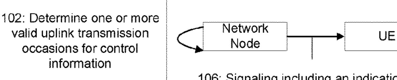
106: Signaling including an indication of a position of a valid uplink transmission occasion for control information relative to a position of one or more other valid uplink transmission occasions for control information
