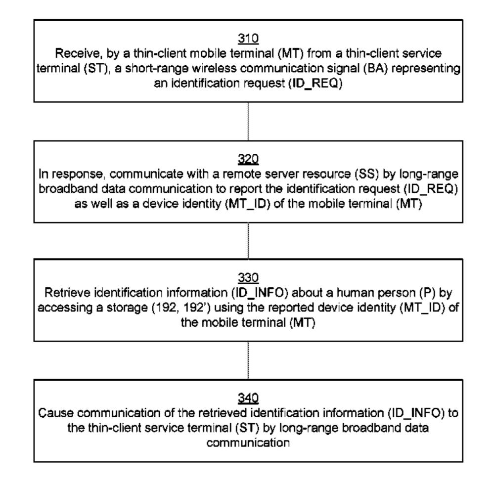
(ID\_INFO) about a human person (P) by accessing a storage (192, 192'), and causing communication communication (104; 106) of the retrieved identification information (ID\_INFO) to the thin-client service terminal (ST) by long-range broadband data communication.
