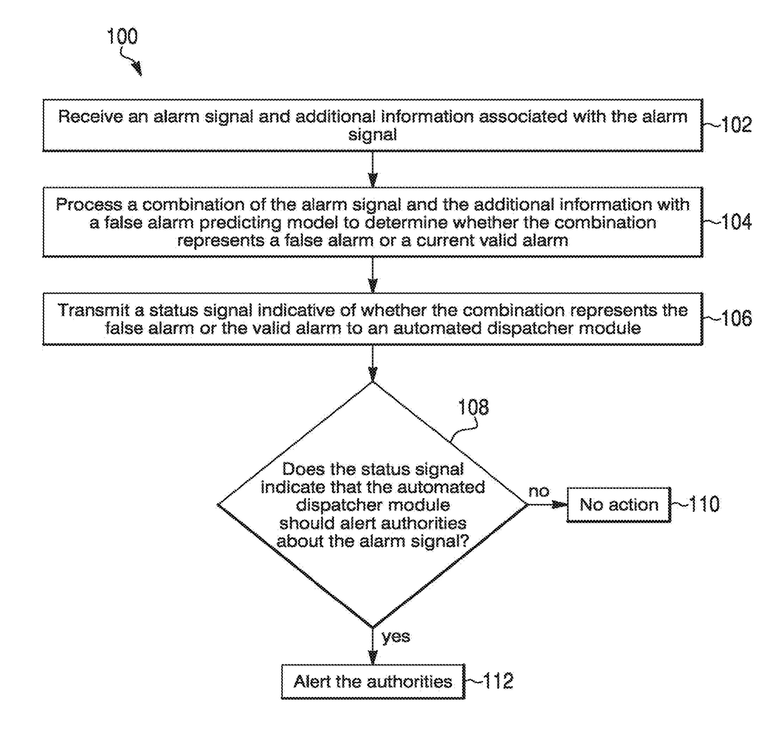
SYSTEMS AND METHODS FOR BUILDING AND USING A FALSE ALARM PREDICTING MODEL TO DETERMINE WHETHER TO ALERT A USER AND/OR RELEVANT AUTHORITIES ABOUT AN ALARM SIGNAL FROM A SECURITY SYSTEM
