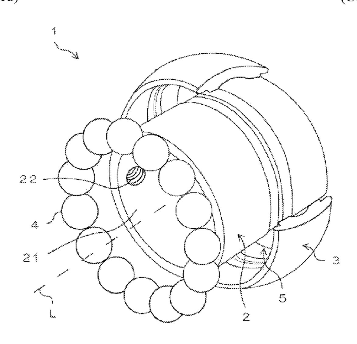
direction, thereby forming an annular second build-up layer with which the plurality of balls contacts so that the balls can be rolled in the circumferential direction (second build-up layer formation step).
