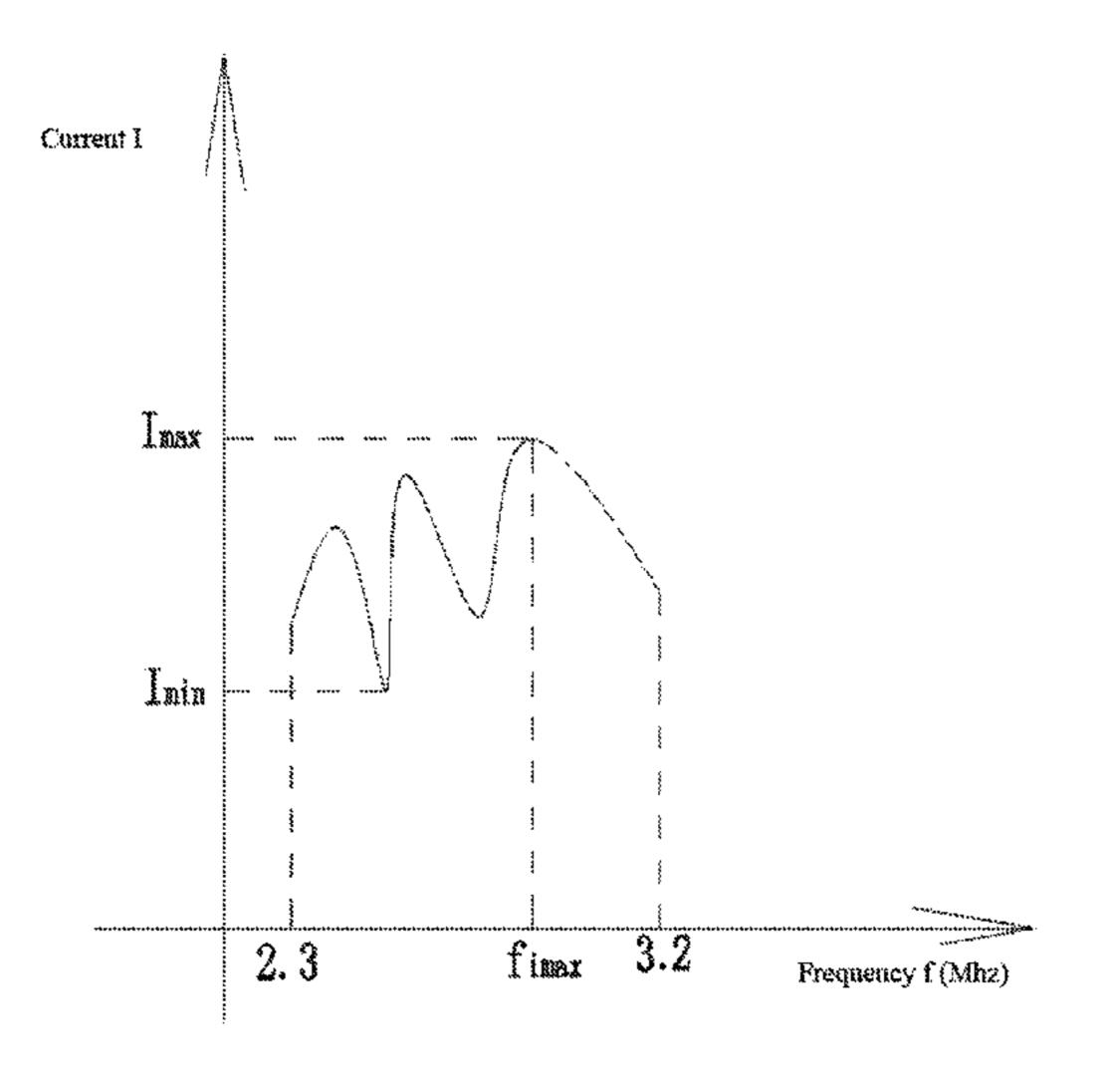
corresponding to the maximum current value Imax. The method further includes controlling the ultrasonic atomizer to work at a frequency  $f_{tracking}$ =fimax+ $\Delta f$ ; and detecting the working current I of the ultrasonic atomizer.
