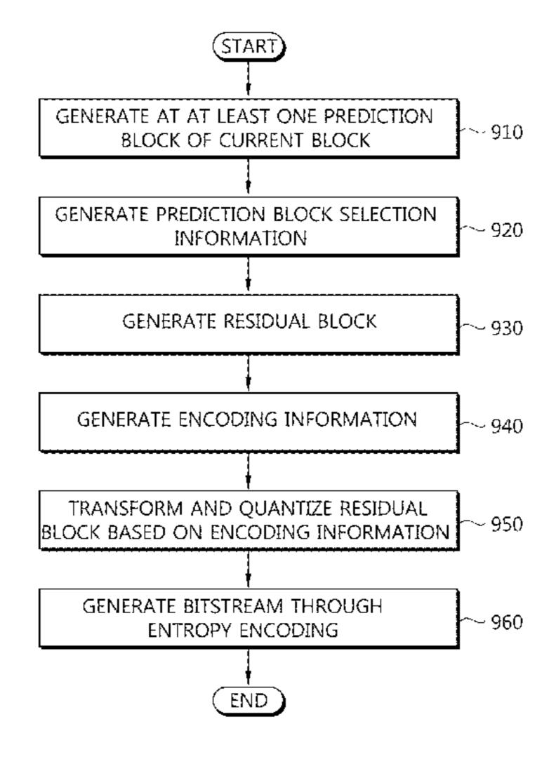
ating a prediction block of a current block according to one of methods for generating a plurality of predetermined prediction blocks, and outputting at least one of encoding information and differential blocks as bitstream by entropy encoding according to whether differential blocks are encoded or not.
