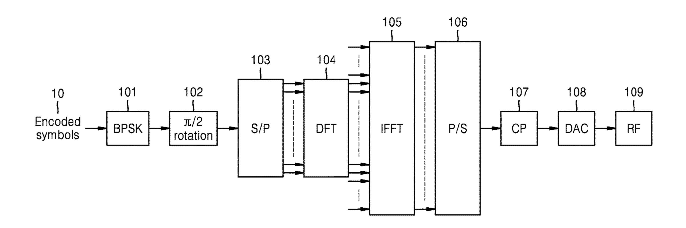
been performed, wherein a constellation of the M symbols on which the  $\pi/2$ -BPSK modulation has been performed may have only real components or imaginary components.
