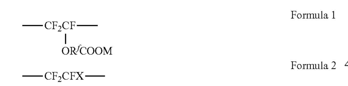
wherein in the formula 1, Rf is a perfluoroperfluoroal-kylene group having 1 to 6 carbon atoms, and M is an alkali metal ion or an ammonium ion, and in the formula 2, X is a fluorine atom or a chlorine atom.
