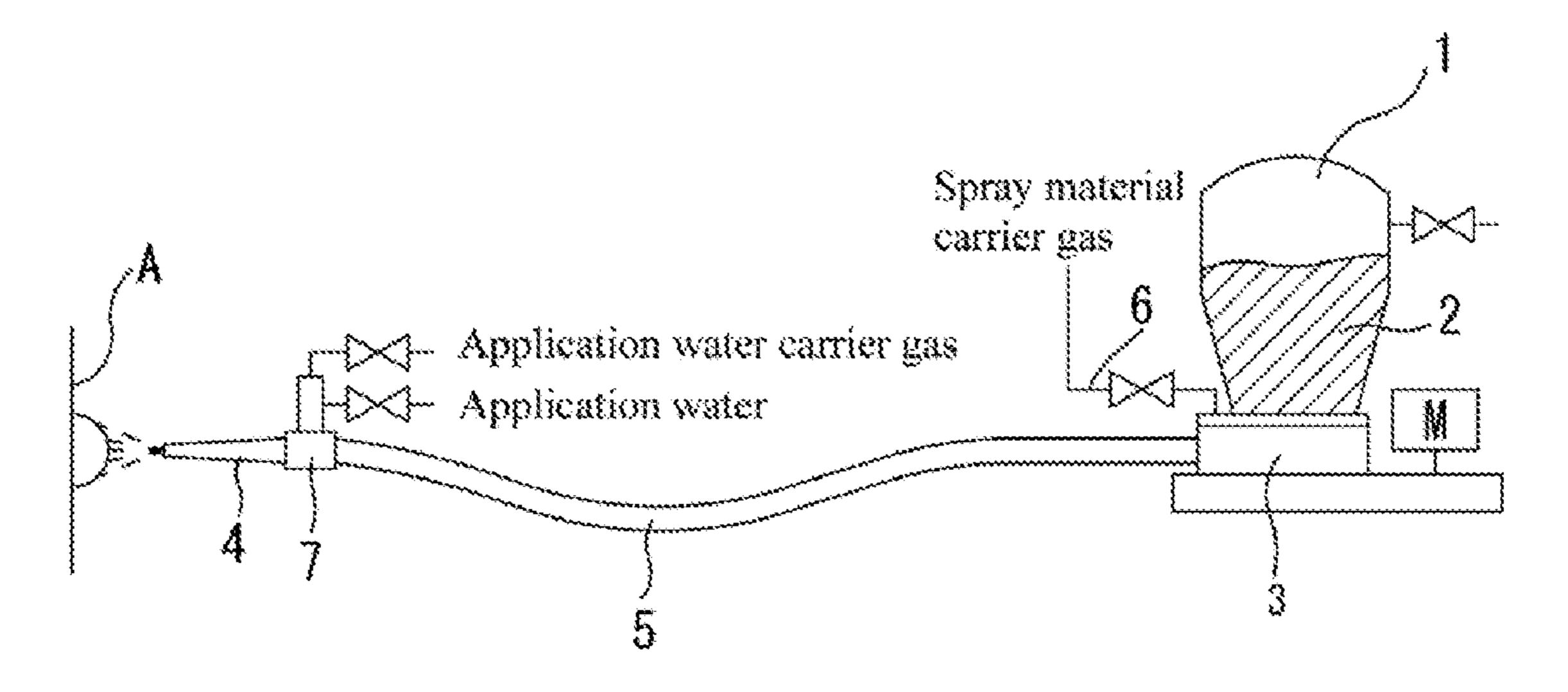
material is set to 0.07 to 2, and a compressibility index of the spray material is set to 32% or less. Alternatively, a ratio of a flow volume of an application water carrier gas for carrying the application water to be introduced into the water injector to an application water volume is set to 100 to 1,000.
