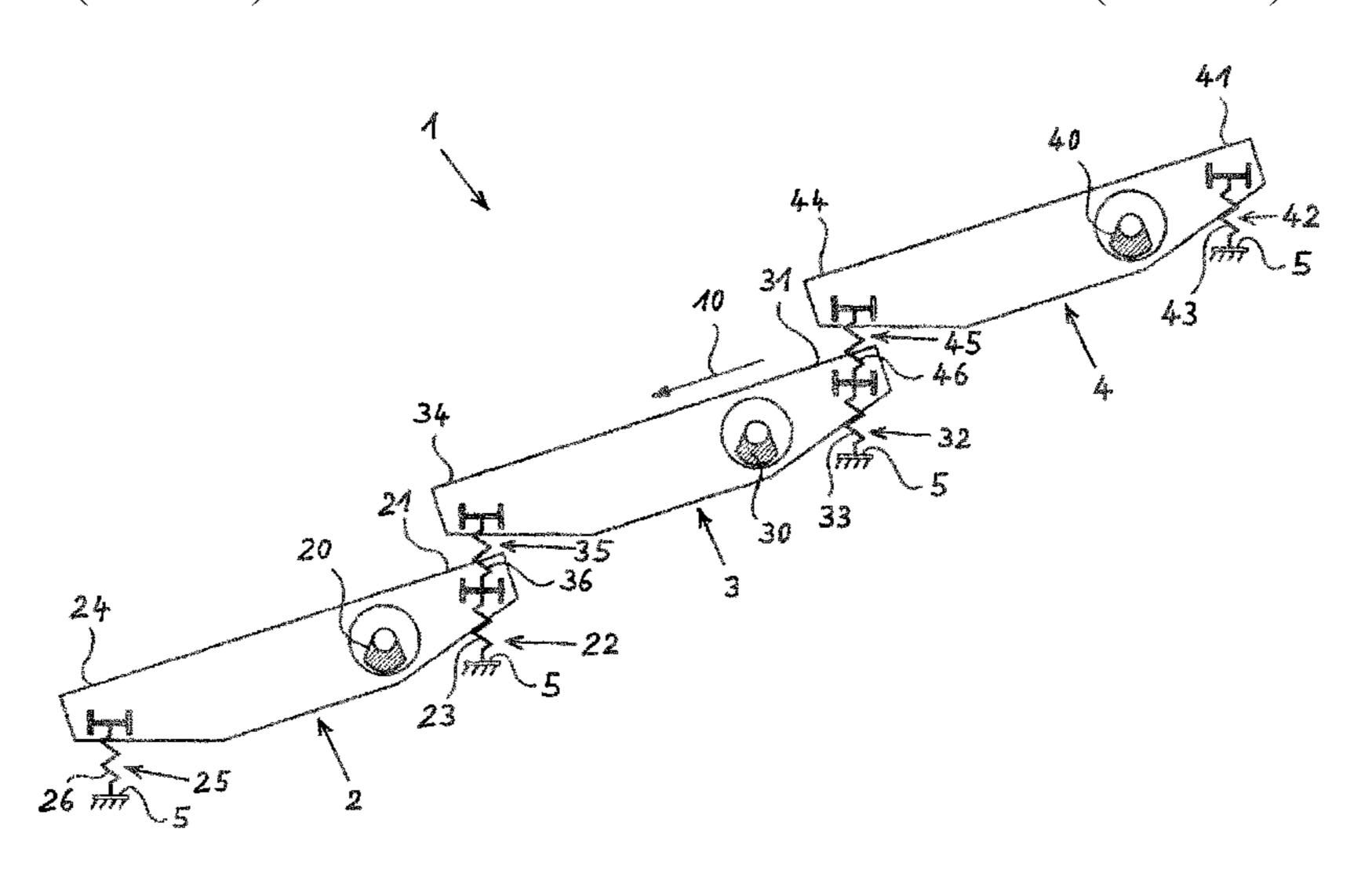
end of any such earlier screening machine in the conveying direction is supported in the region of the screening material feed end of the screening machine that is subsequent in the screening material conveying direction, on this subsequent machine.
