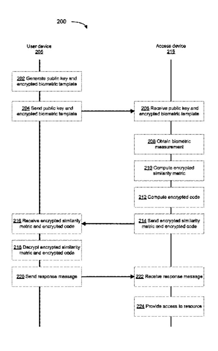
matches a test code. The second device can then authenticate the user based on the response.
