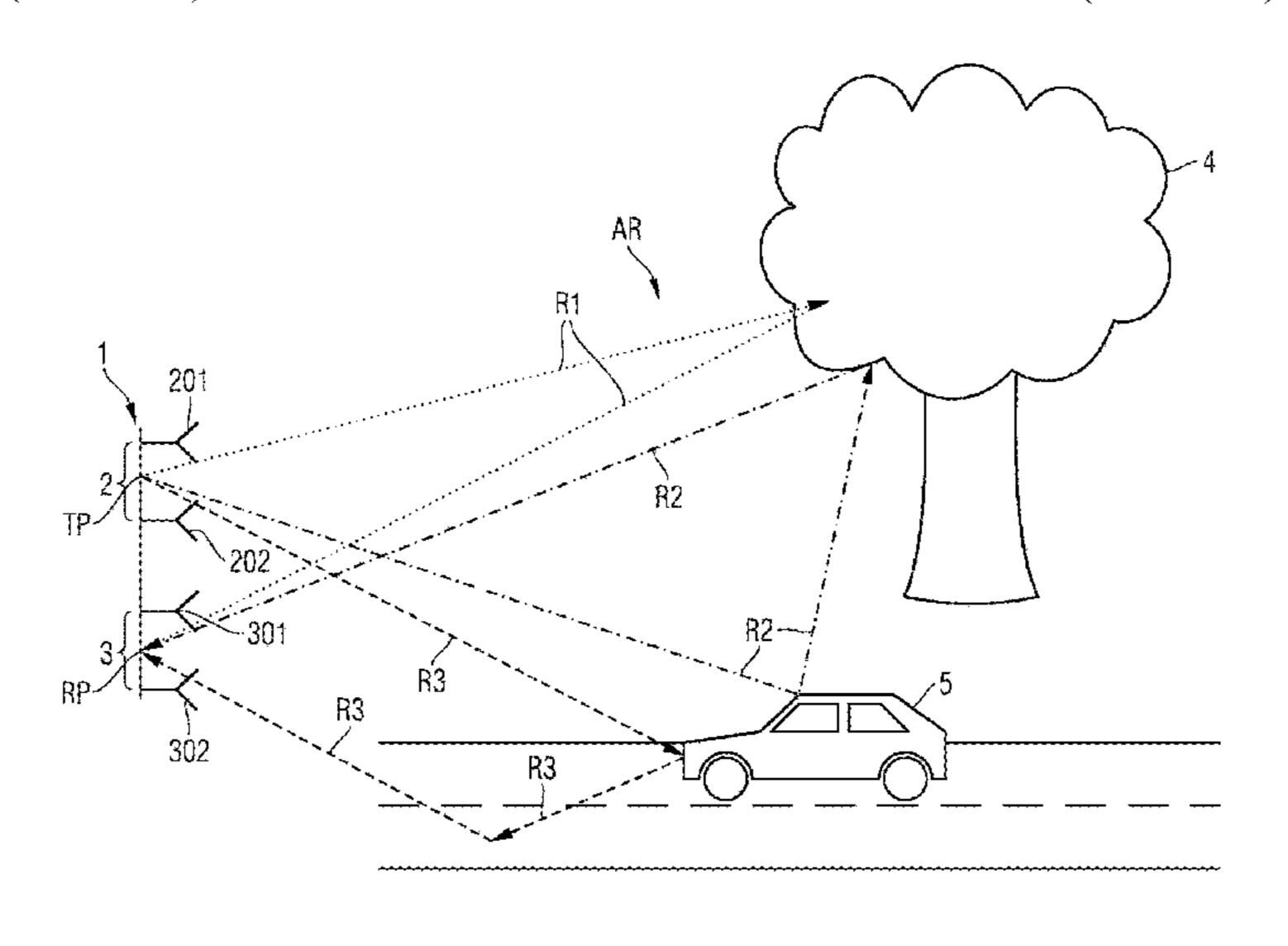
first angle and the second angle, propagations of a plurality of modified rays originating from a respective transmitter and received at a respective receiver are determined based on a linear approximation. The modified rays are processed in order to determine the radar raw data.
