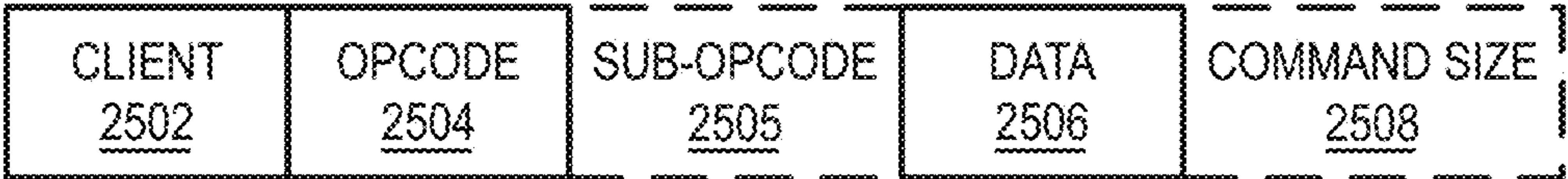
FIG. 25A GRAPHICS PROCESSOR COMMAND FORMAT 2500
