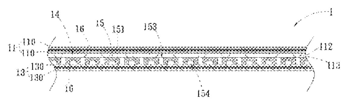
multiple perforations and multiple channels. The multiple perforations pass through the first and second faces. The multiple channels are disposed on one of the first and second faces. By means of the above arrangement, the total thickness of the vapor chamber structure is equal to or smaller than 0.25 mm, whereby the vapor chamber can be extremely thinned.
