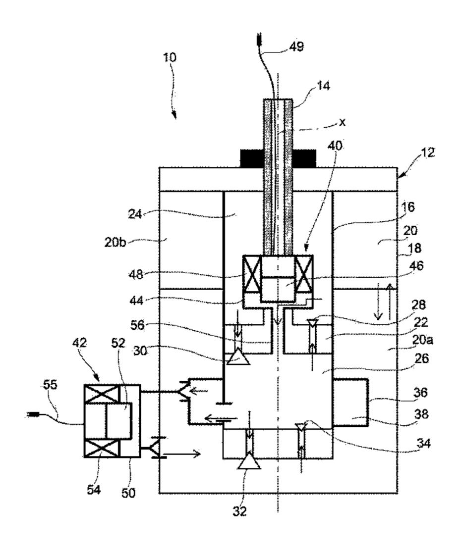
chamber. A second electronically-controlled valve is arranged outside the cylindrical body and is hydraulically connected to the reservoir chamber and to the intermediate chamber to adjust, during compression phase, flow of the damping fluid from the compression chamber to the reservoir chamber via the intermediate chamber.
