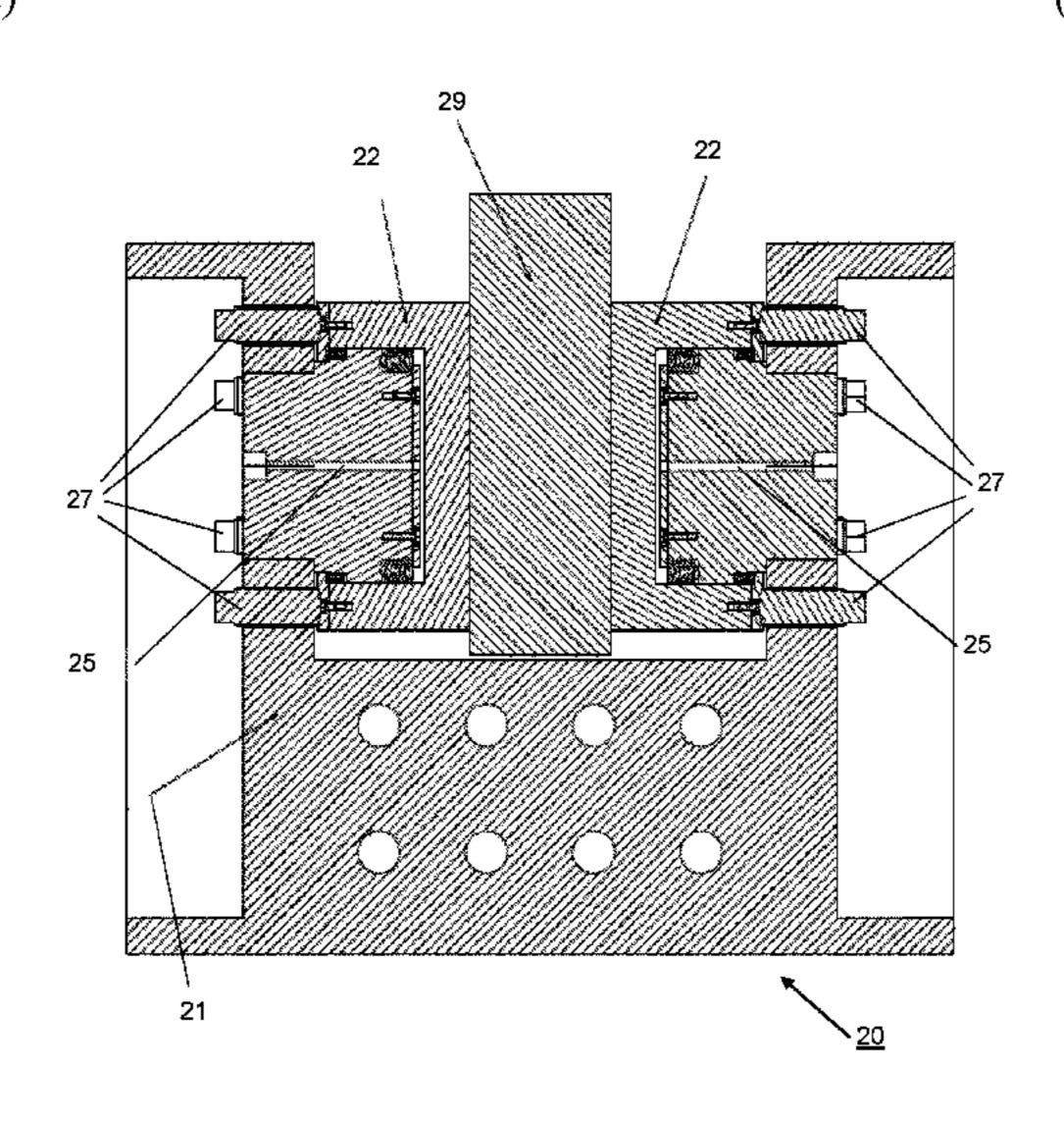
against the brake disk creates a micro-interference fit between the at least one brake block and the brake disk.
