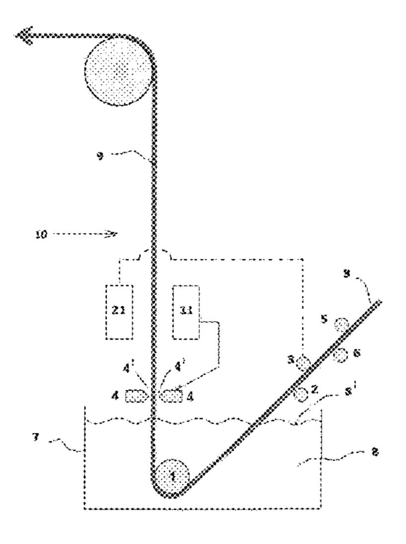
use, having an outlet to project wiping gas on the metal coating on the metal sheet. At least one supporting roll with the guide or sink roll in use influence metal sheet shape in its width direction at the gas knife location. The one supporting roll is above liquid bath surface level to operate on the metal sheet before the metal sheet enters the bath. A method for use of the device.
