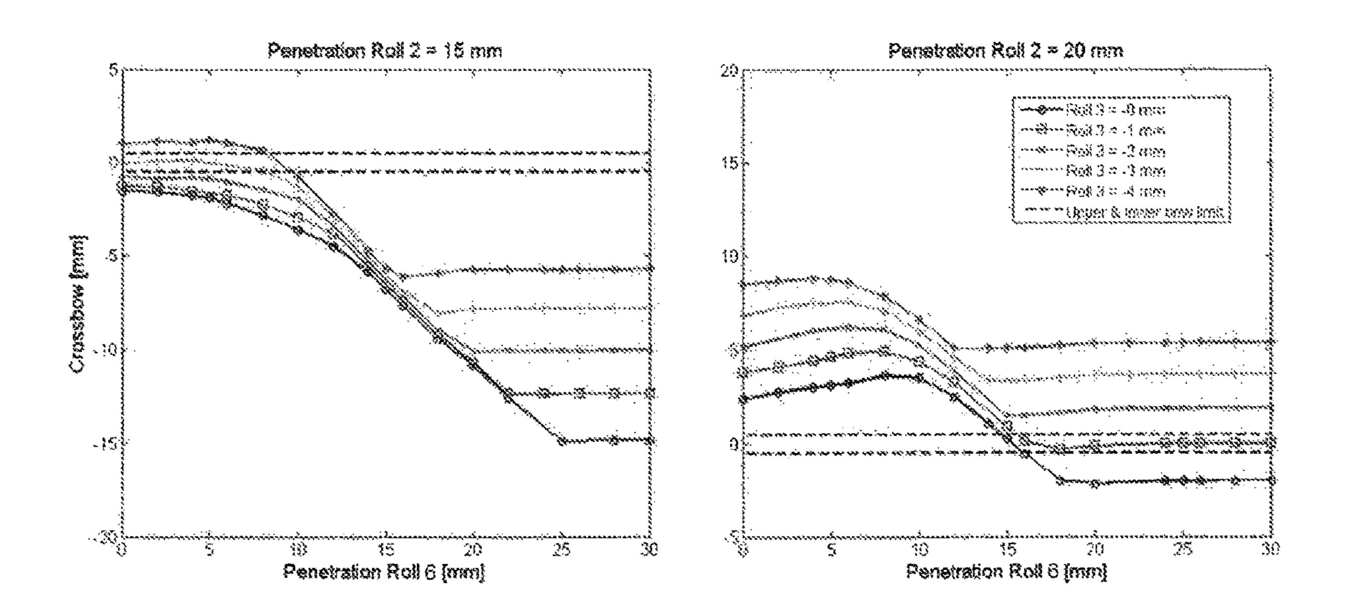
Fig.5. Crossbow for different settings in the configuration of figure 3.
