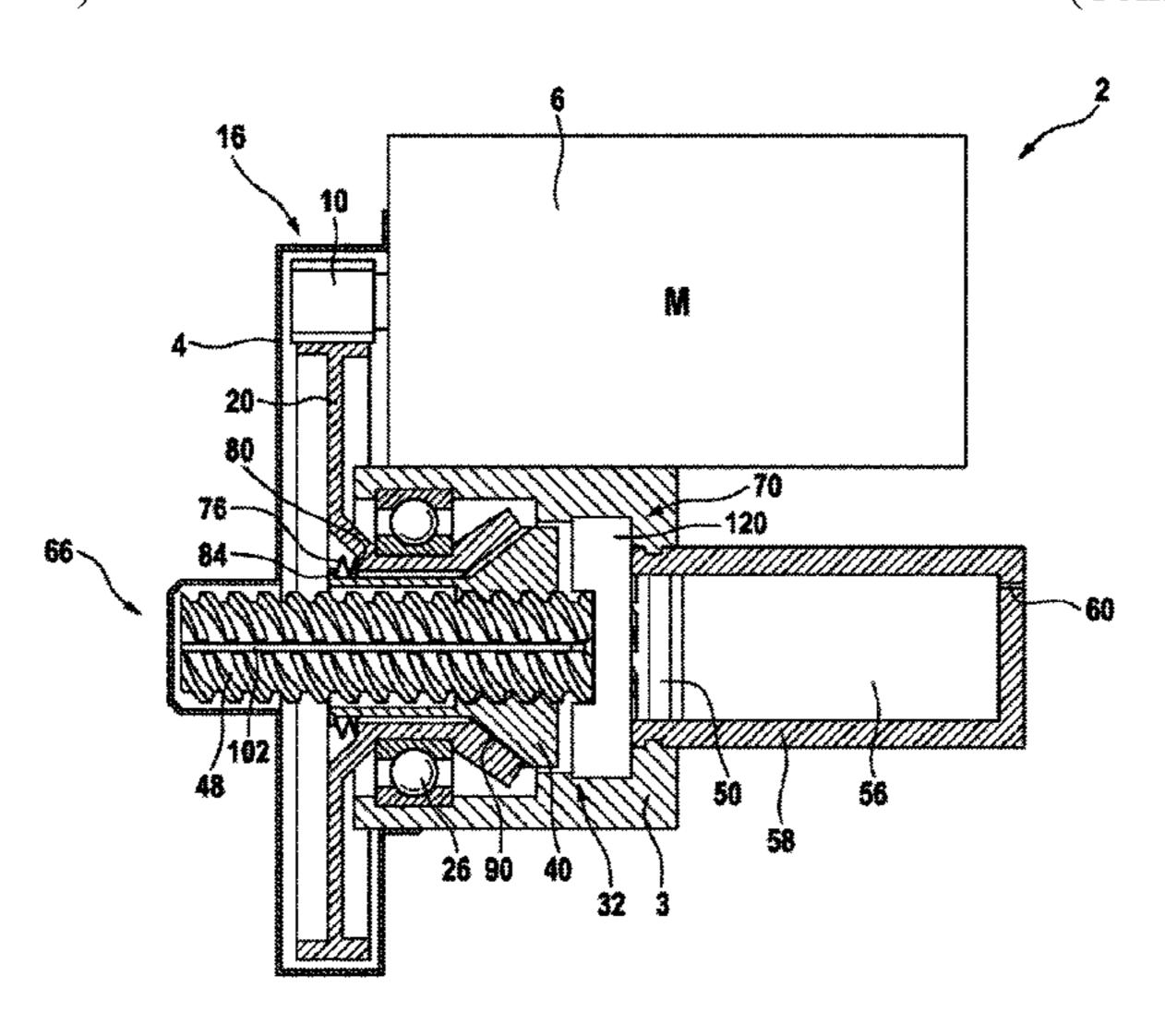
for the piston-travel-controlled isolation of the rotational coupling between the rotor of the electric motor and the threaded nut.
