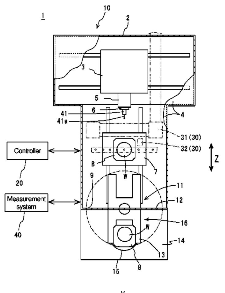
adjusting means (30) used in machining of the workpiece (W) to adjust an ambient temperature of the machining area.
