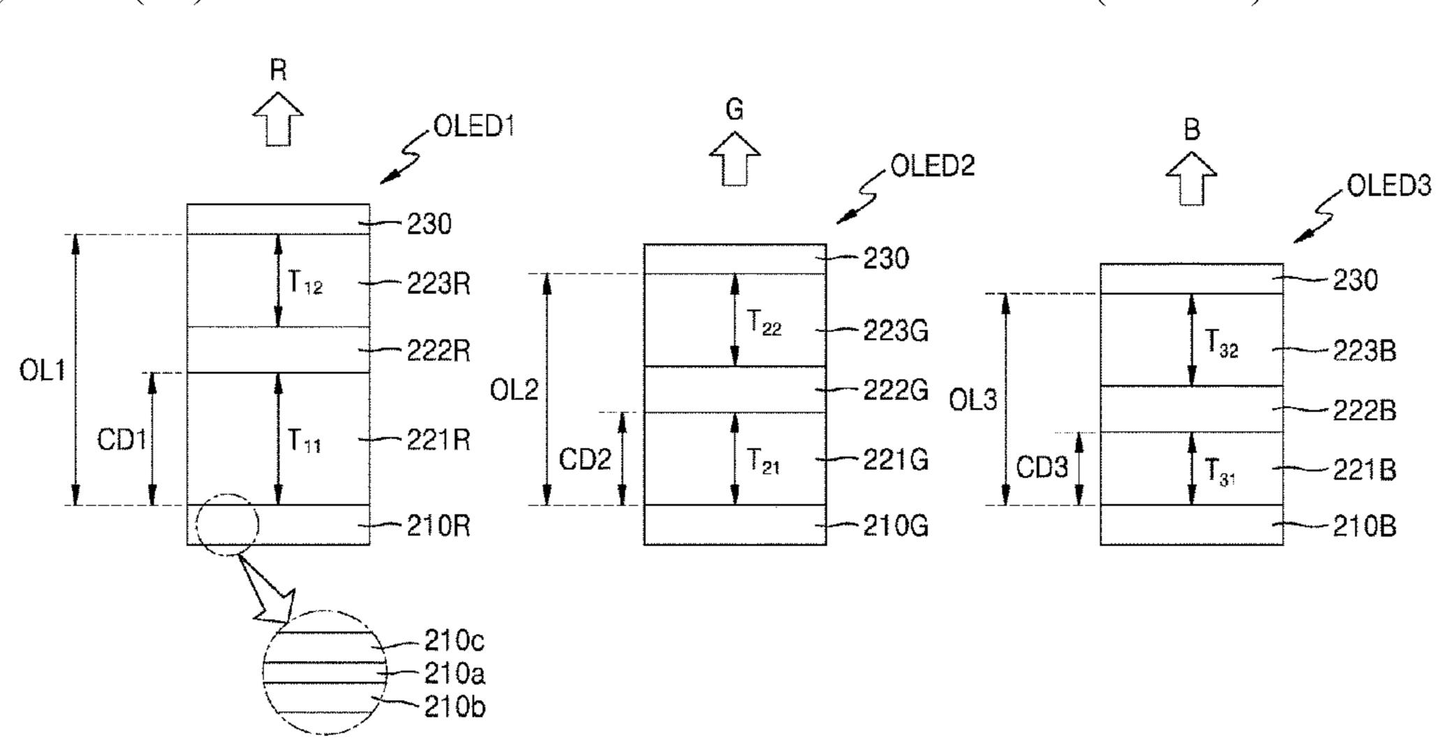
layer respectively disposed between the opposite electrode and the first organic emission layer, the second organic emission layer, and the third organic emission layer and each having a thickness that is equal to or greater than about 1300 Å and less than or equal to about 1800 Å.
