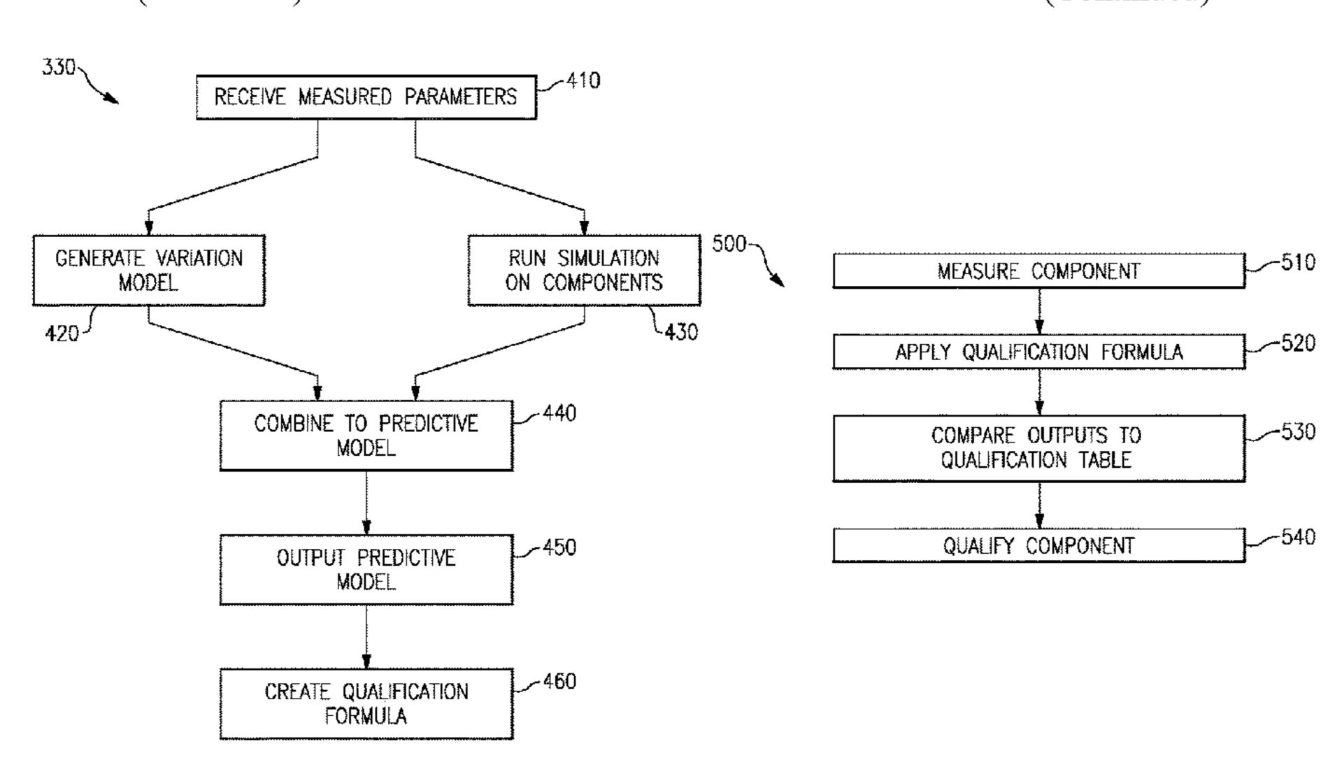
component and determine when the as manufactured gas turbine engine component is qualified for inclusion in at least one engine.
