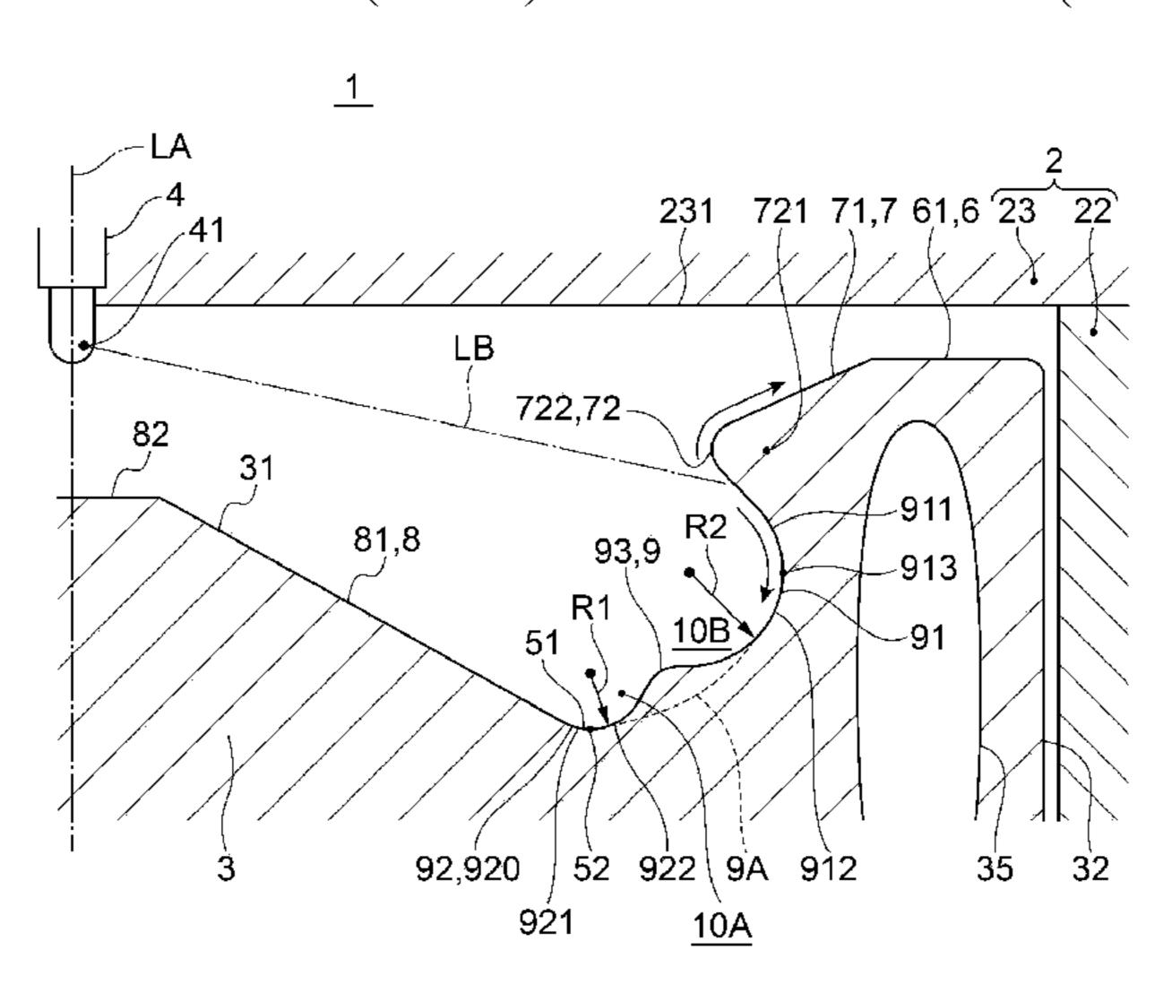
the cavity, and a convex surface formed between the outer circumference-side curved surface and the inner circumference-side concave surface, as well as protruding upward.
