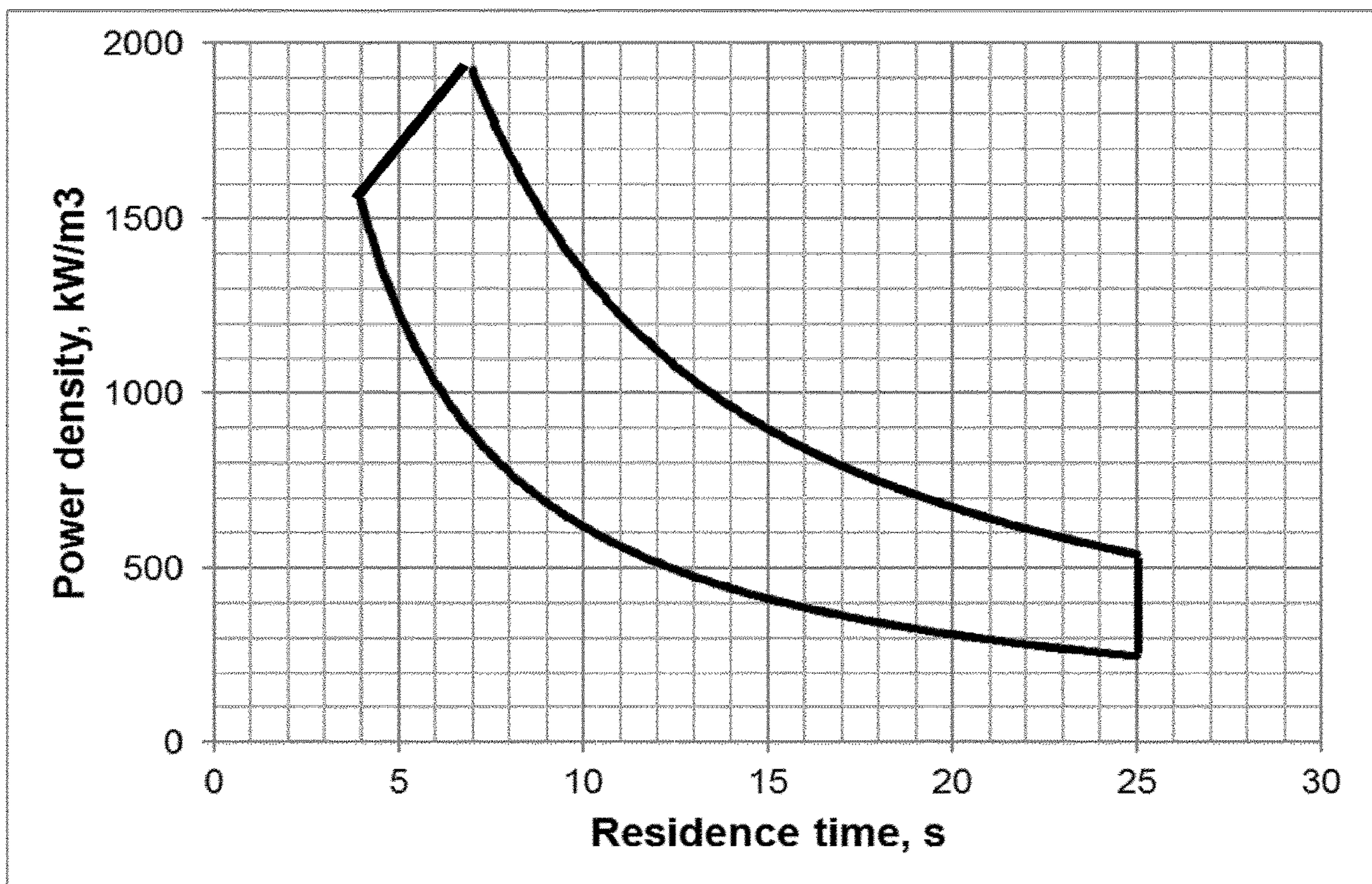
Fig. 6. A preferred range of power density vs. the residence time in the homogenizer.
