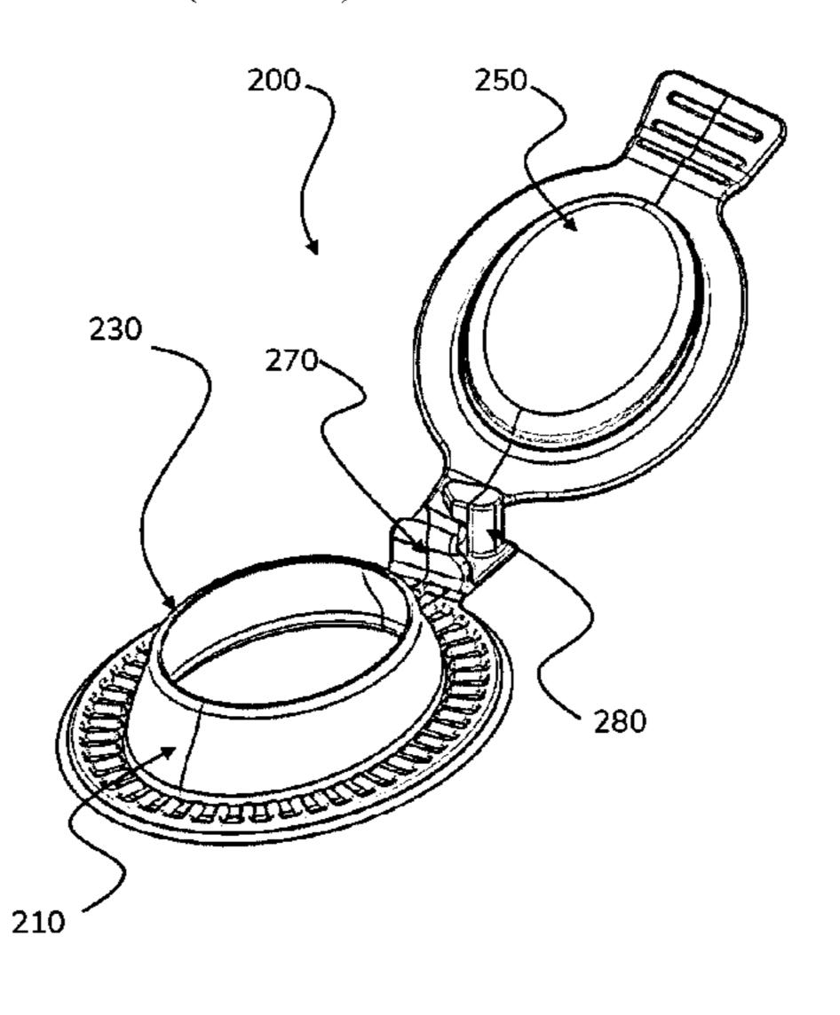
portion is a flexure hinge allowing the lid portion to pivot away from the base portion after the breakable sealing portion has been broken.
