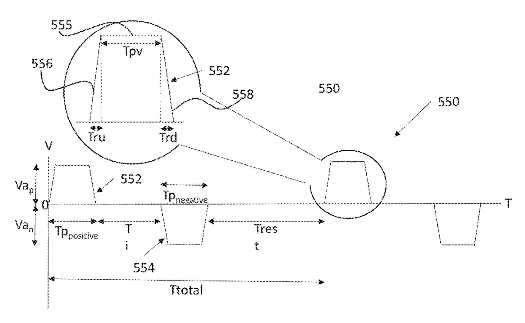
fulfills at least one of the following structural conditions: (1) the positive voltage pulse attains at least 80% of the time-averaged voltage amplitude, within a time (T80) of 70-150 nanoseconds; (2) the positive voltage pulse increases by at least 20 Volts, within 70 nanoseconds.
