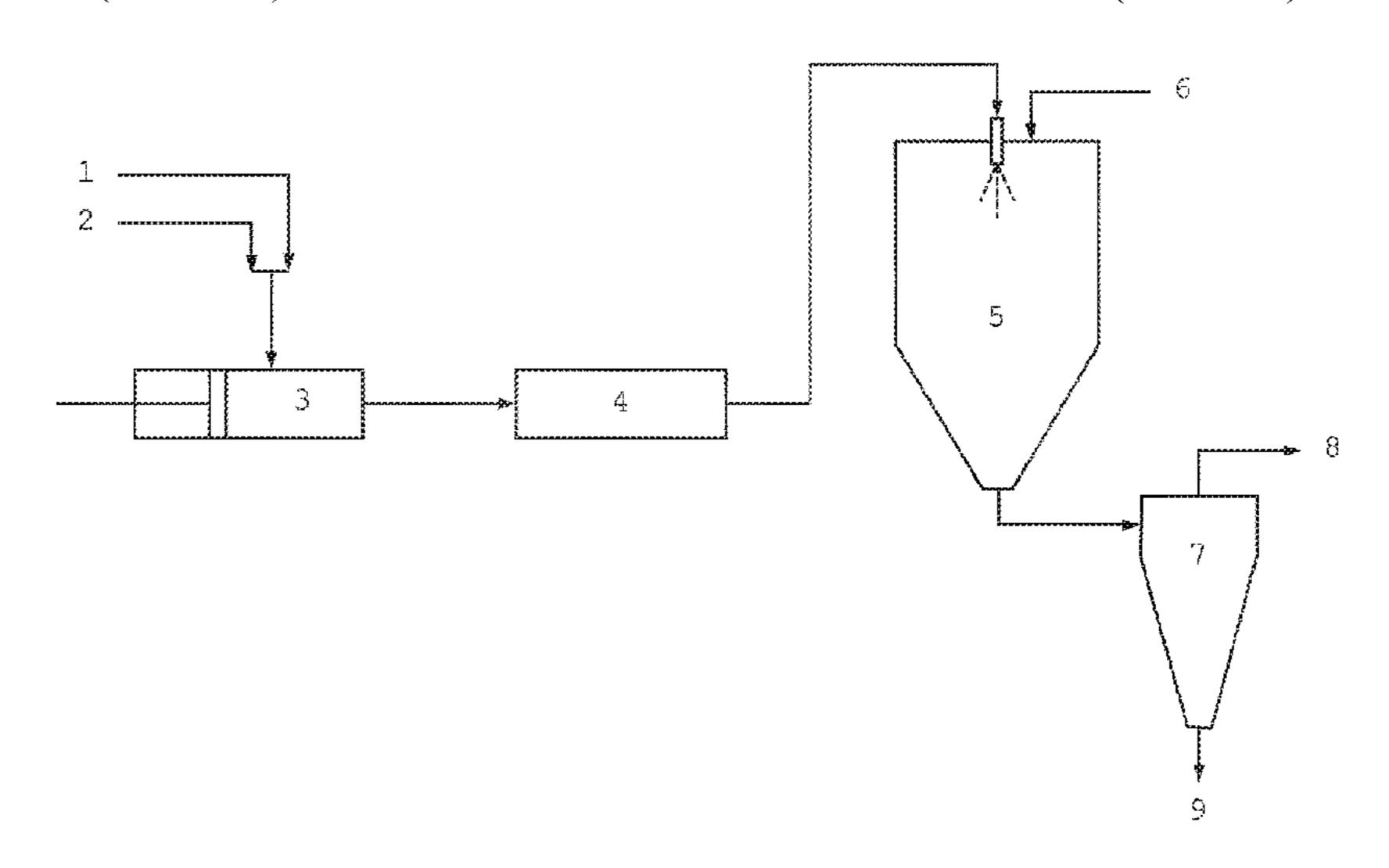
ously fed to the spray dryer through at least one atomization nozzle, drying said atomized stream to obtain solid particles and collecting said solid particles. Single component particles or multi-component particles, particulate amorphous solid dispersion and pharmaceutical compositions are also disclosed. The present invention also discloses amorphous solid dispersions obtained by the method of the invention as well as pharmaceutical compositions containing the same.
